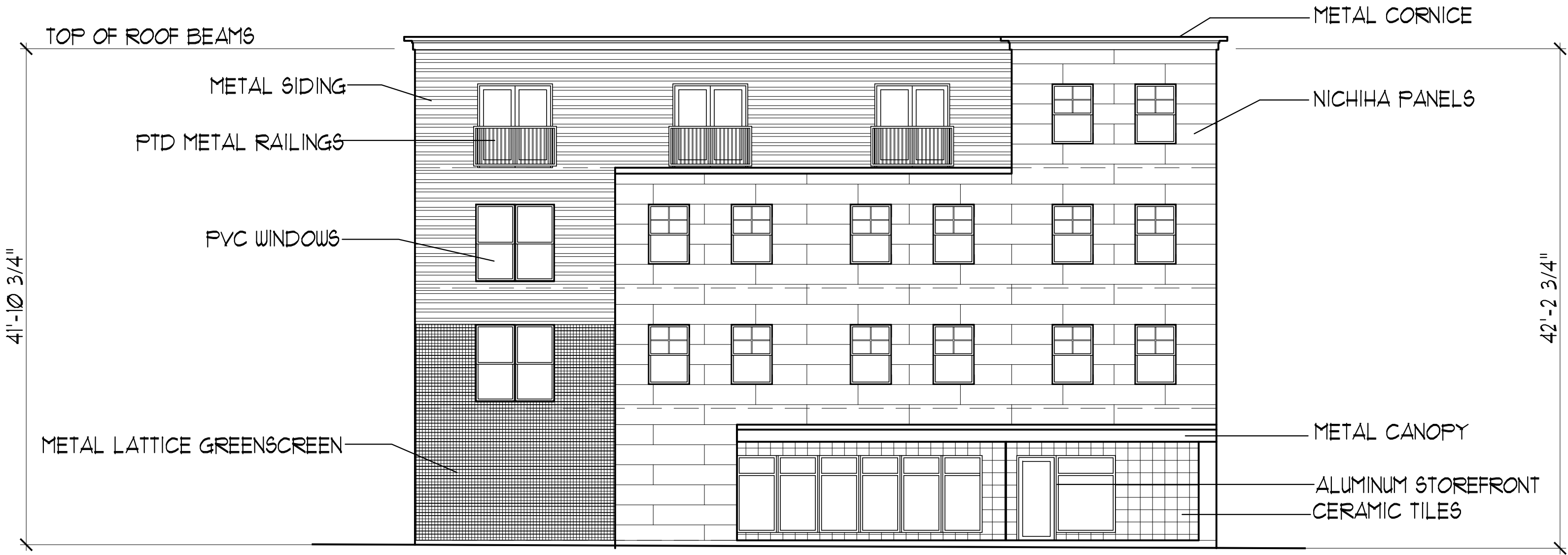
EAST ELEVATION - WASHINGTON AVENUE
