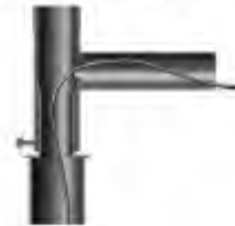
Pole Top Bracket Attachment
