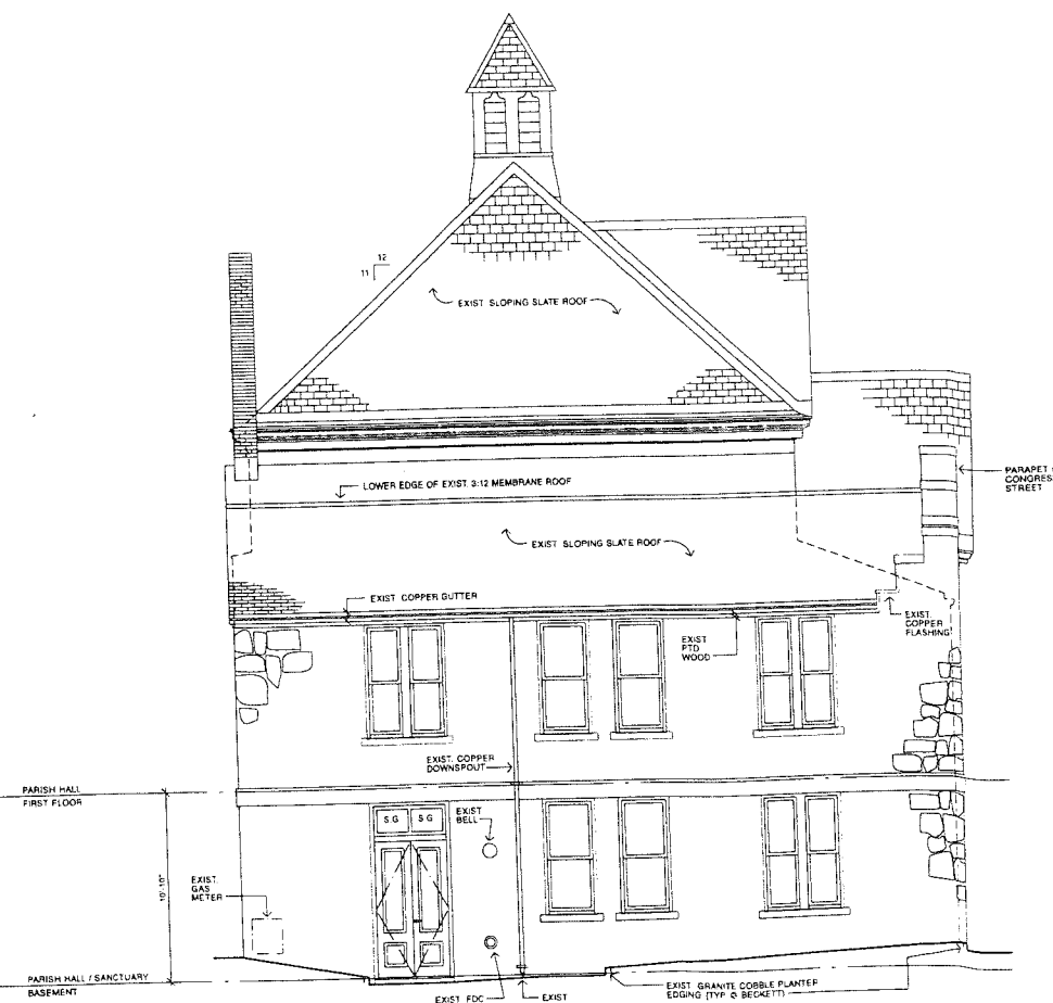
2 PROPOSED EAST EXTERIOR ELEVATION - BECKETT STREET A-13.1
