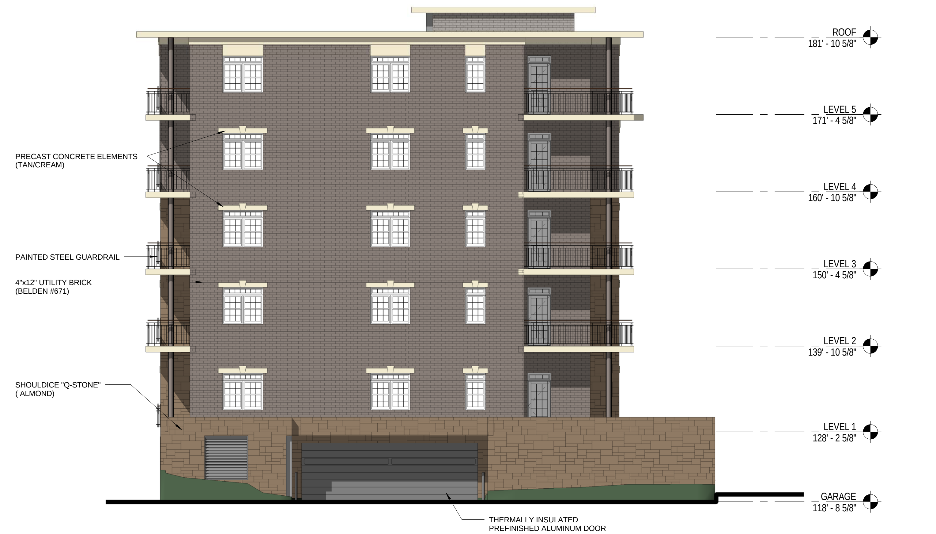
D NEW BUILDING - SOUTHEAST ELEVATION 008 1/8" = 1'-0"
