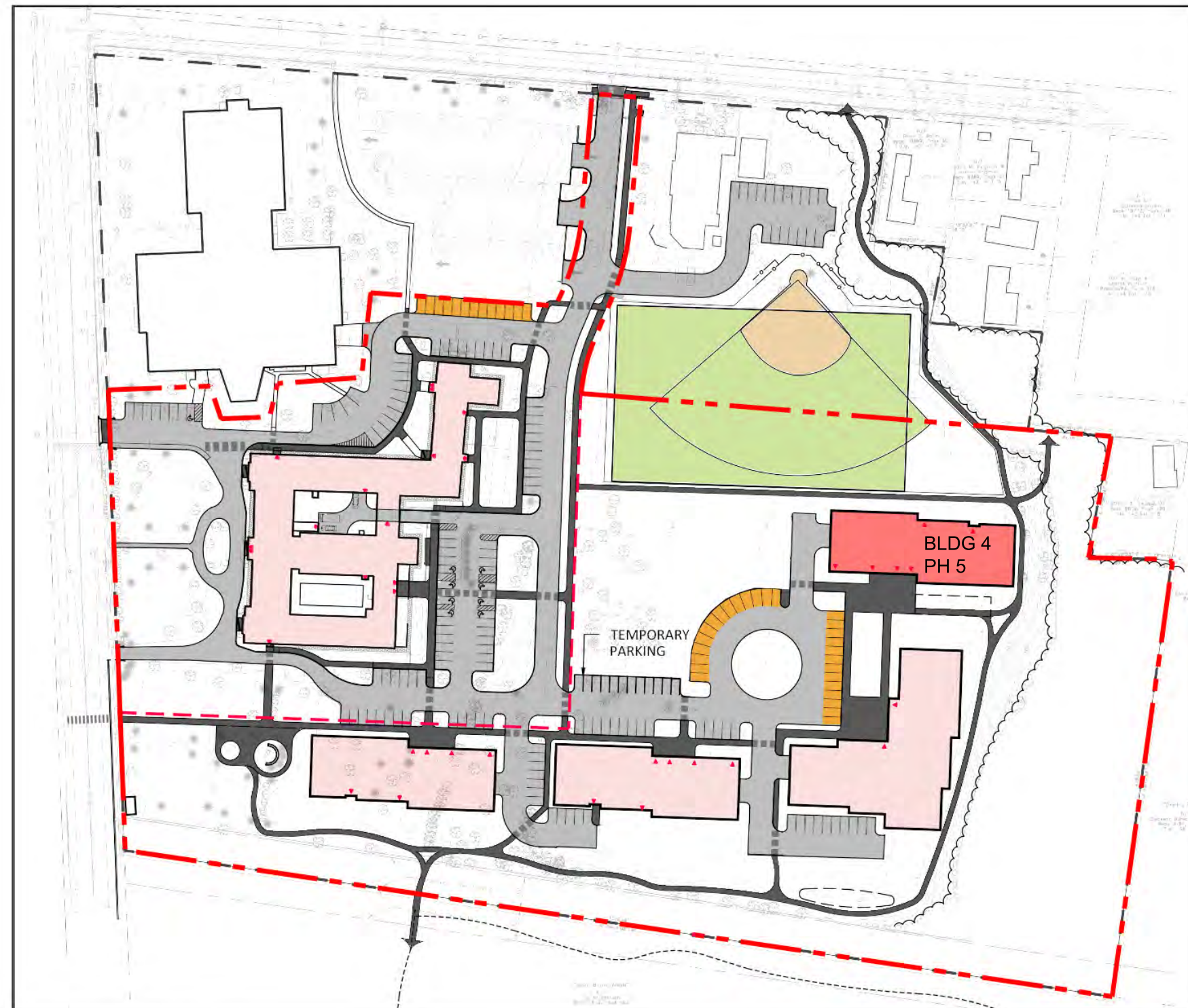
PHASE V BUILDING #4 CONSTRUCTED (28 DU) NEW FIELDS CONSTRUCTED 28 DU 31 COVERED P.S. 25 SURFACE P.S. 173 TOTAL SURFACE 311 TOTAL SPACES
