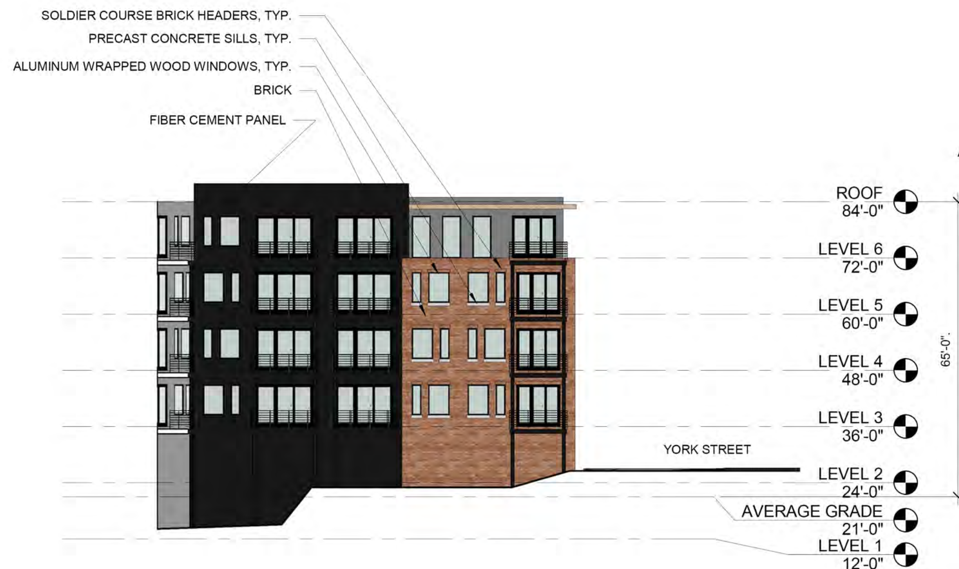
3 | PHASE 1 - EAST ELEVATION 1" = 20'-0"
