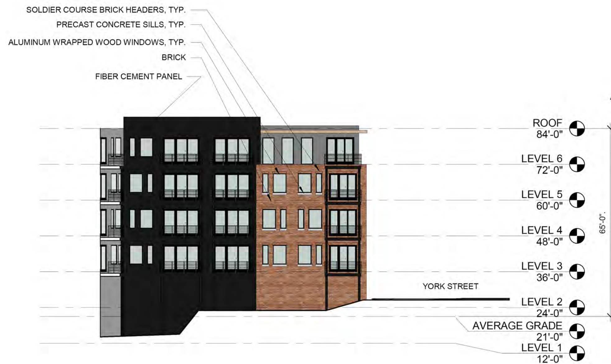
3 | PHASE 1 - EAST ELEVATION 1" = 20'-0"
