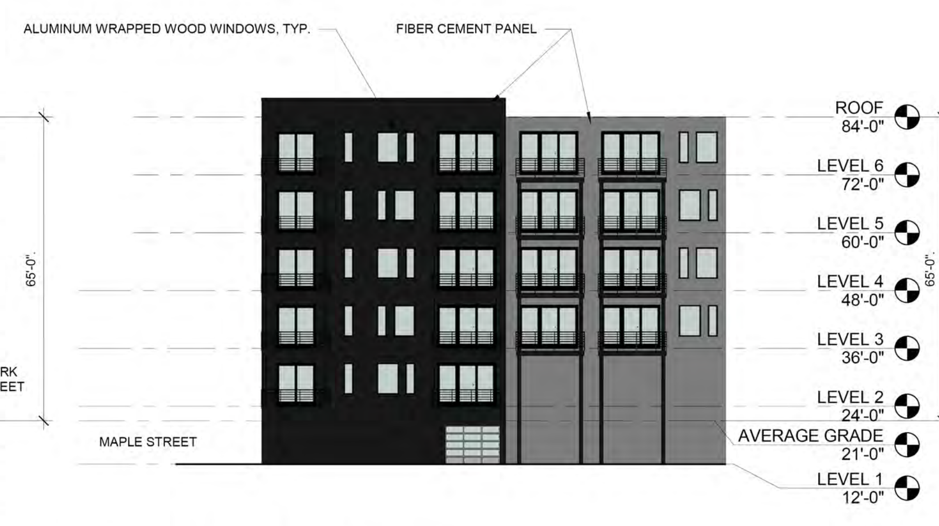
2 | PHASE 1 - WEST ELEVATION 1" = 20'-0"
