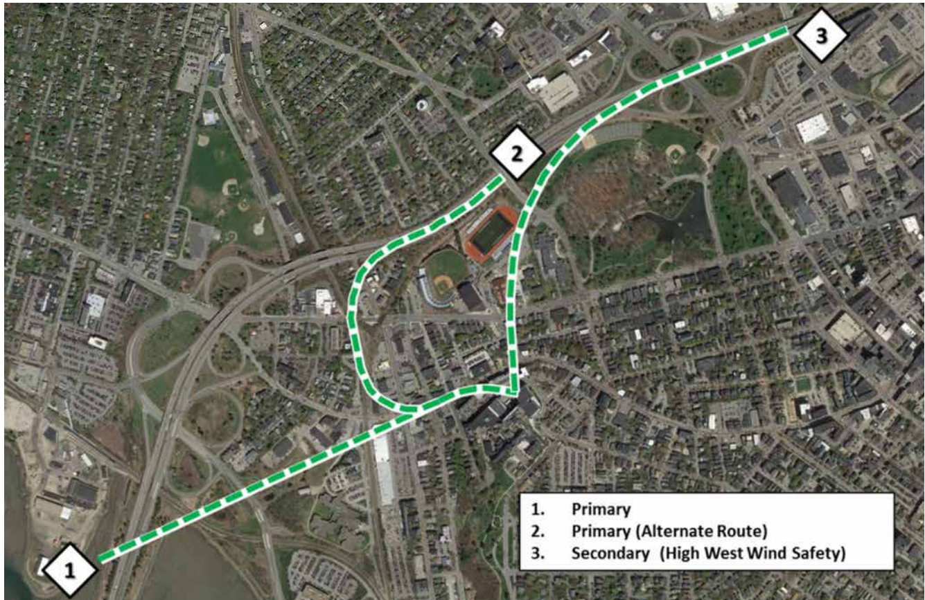
Fig.4.5 Proposed Flight Routes for the new MMC Helipad
