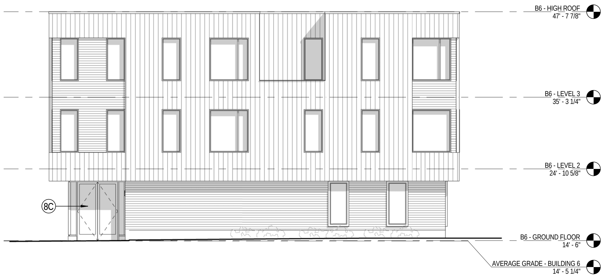
2 BUILDING 6 - EAST ELEVATION 1/8" = 1'-0"
