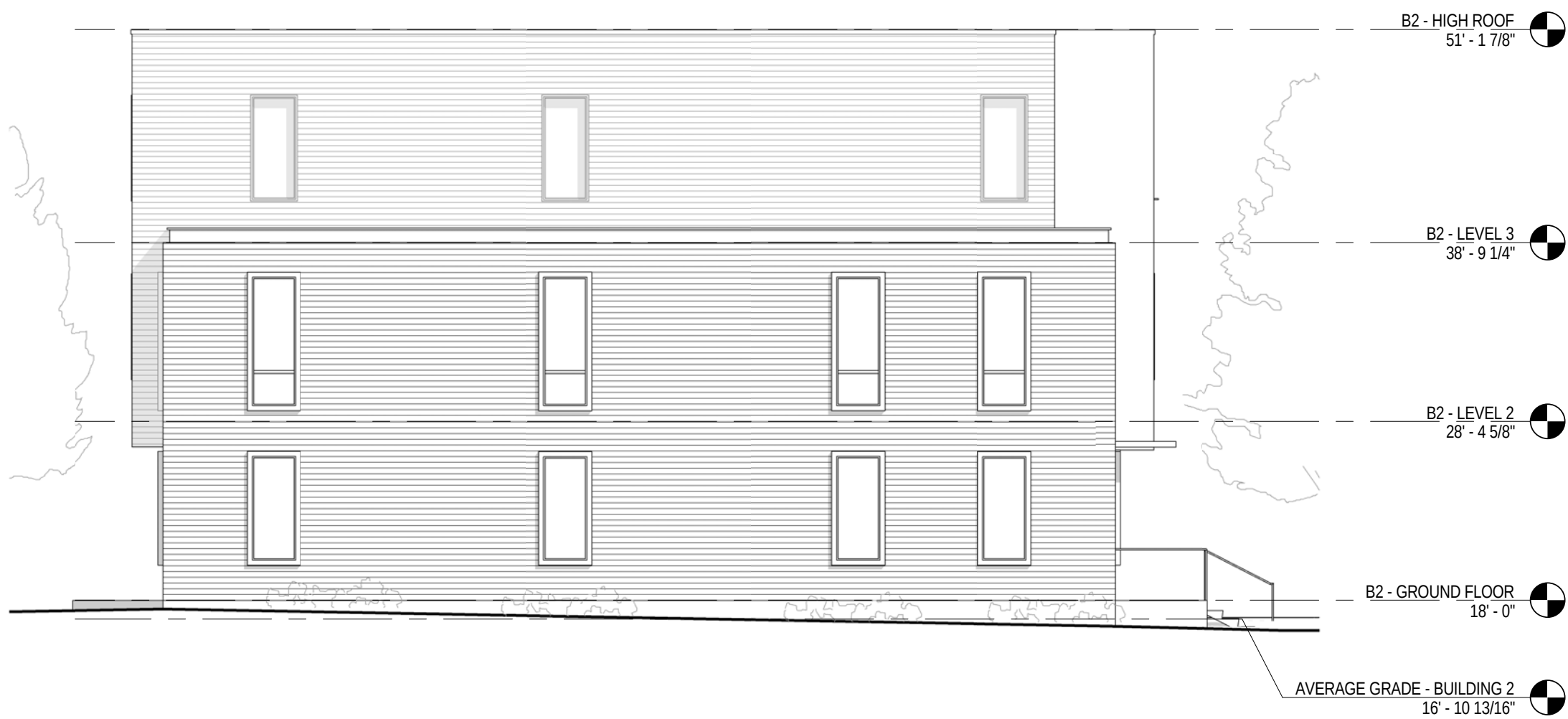
4 BUILDING 2 - EAST ELEVATION 1/8" = 1'-0"
