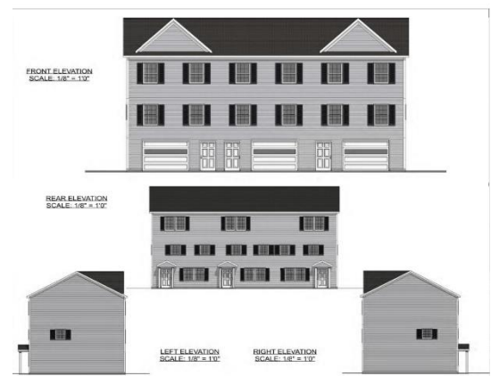
Figure 8: Building elevations - triplex
