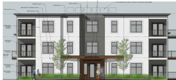
Figure 4: Revised front elevation, note that mechanical equipment is roof-mounted.
