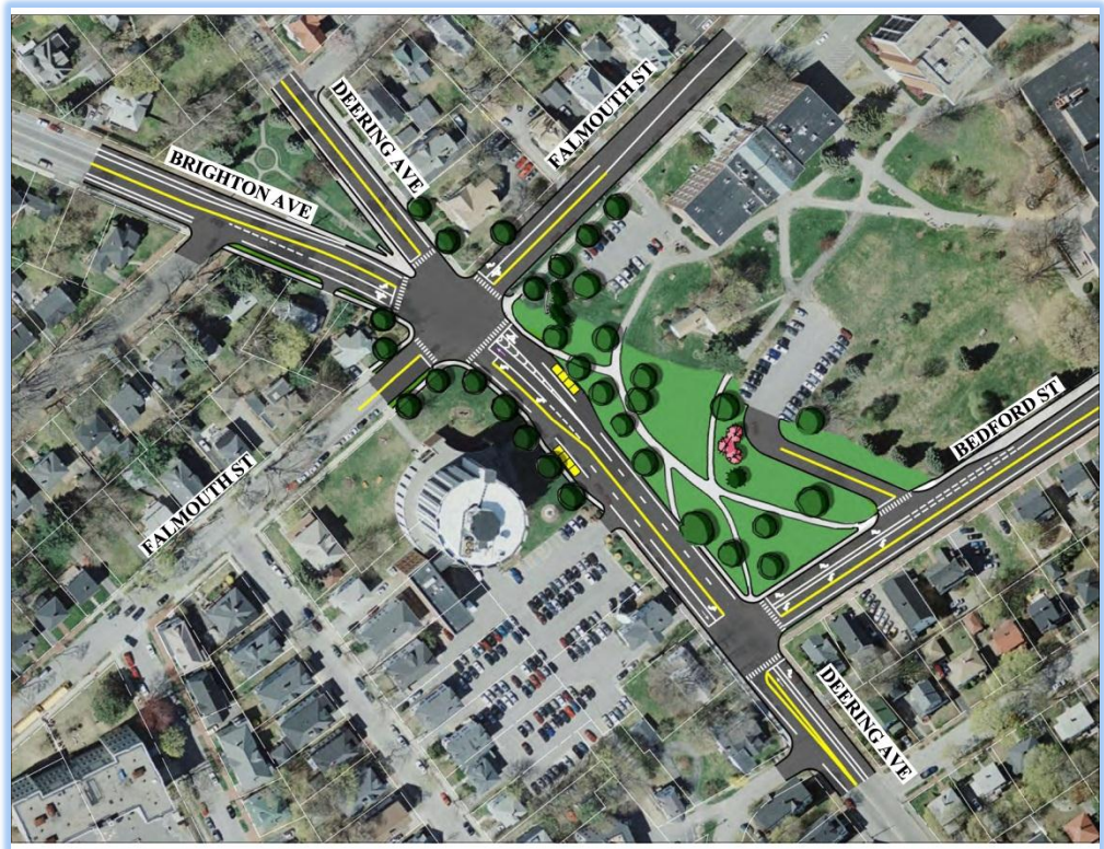
Figure 5 - Signal (Modified) with Bedford St Signal
