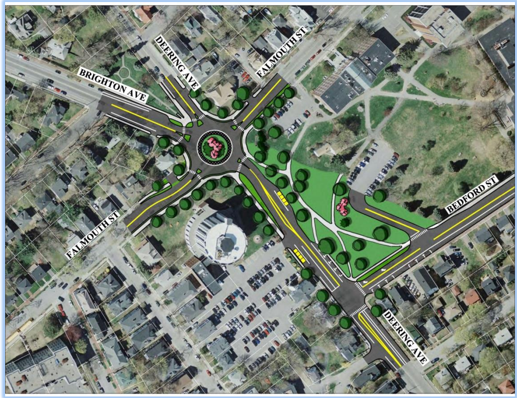
Figure 7 - 5 Leg Roundabout with Bedford St Signal
