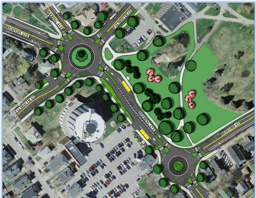
Figure 9 - 5 Leg Roundabout with Full Roundabout
