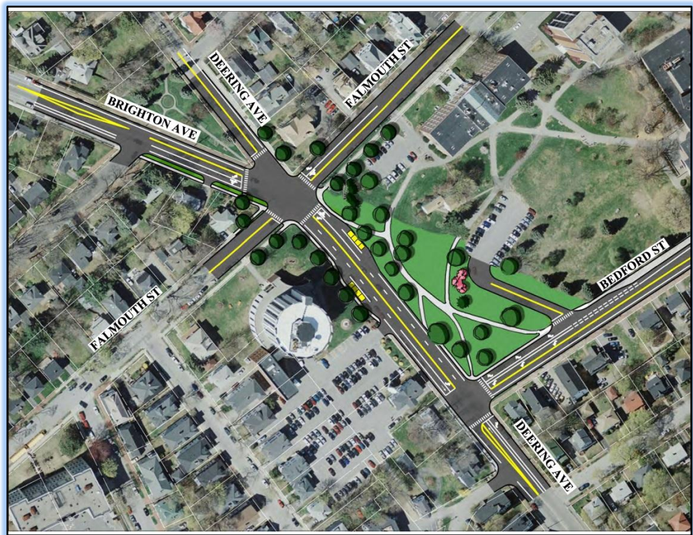
Figure 4 - 5 Leg Signal with Bedford Street Signal
