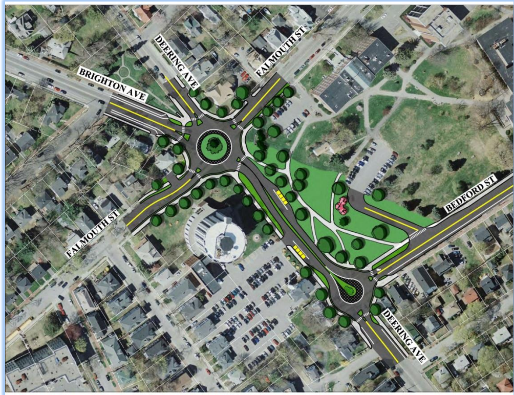
Figure 8 - 5 Leg Roundabout with Mini-Roundabout
