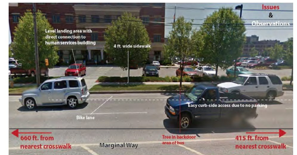
Figure 2-24: Existing conditions at a mid-side stop, located at 161 Marginal Way, formerly the Human Services building
