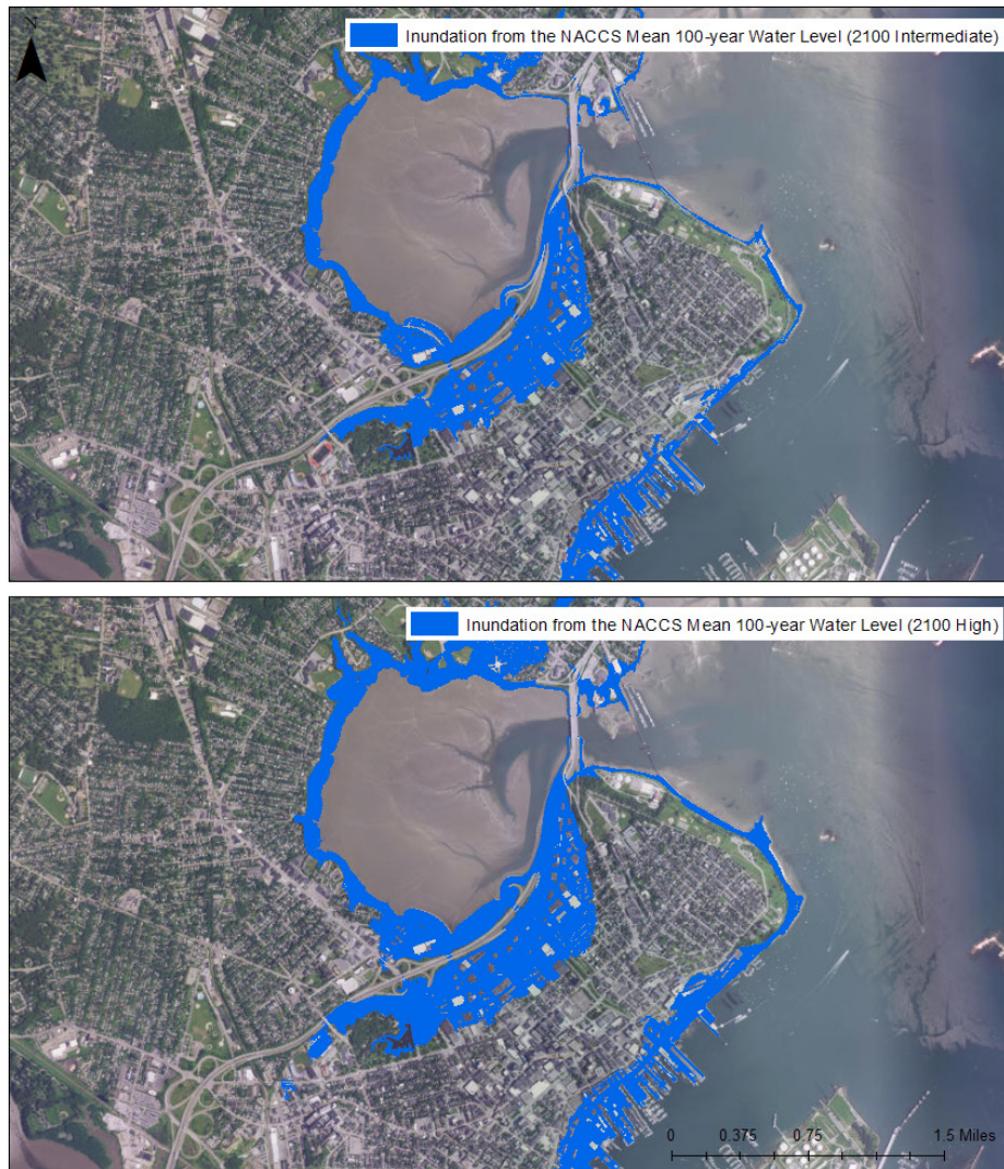
Figure 5-7: Inundation from the NACCS Mean 100-year Storm Surge Water Level for the 2100 Intermediate (top) and High (bottom) Scenarios
