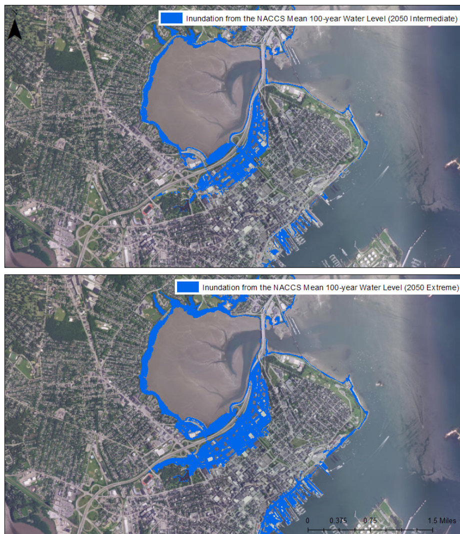
Figure 5-6: Inundation from the NACCS Mean 100-year Storm Surge Water Level for the 2050 Intermediate (top) and Extreme (bottom) Scenarios
