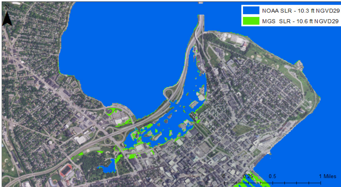
Figure 5-5: Comparison of Inundation Extent Layers from NOAA SLR Viewer and the MGS SLR/Storm Surge Viewer
