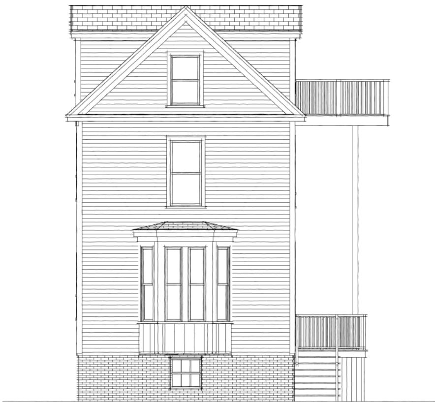
West Elevation (Deck on Posts)
