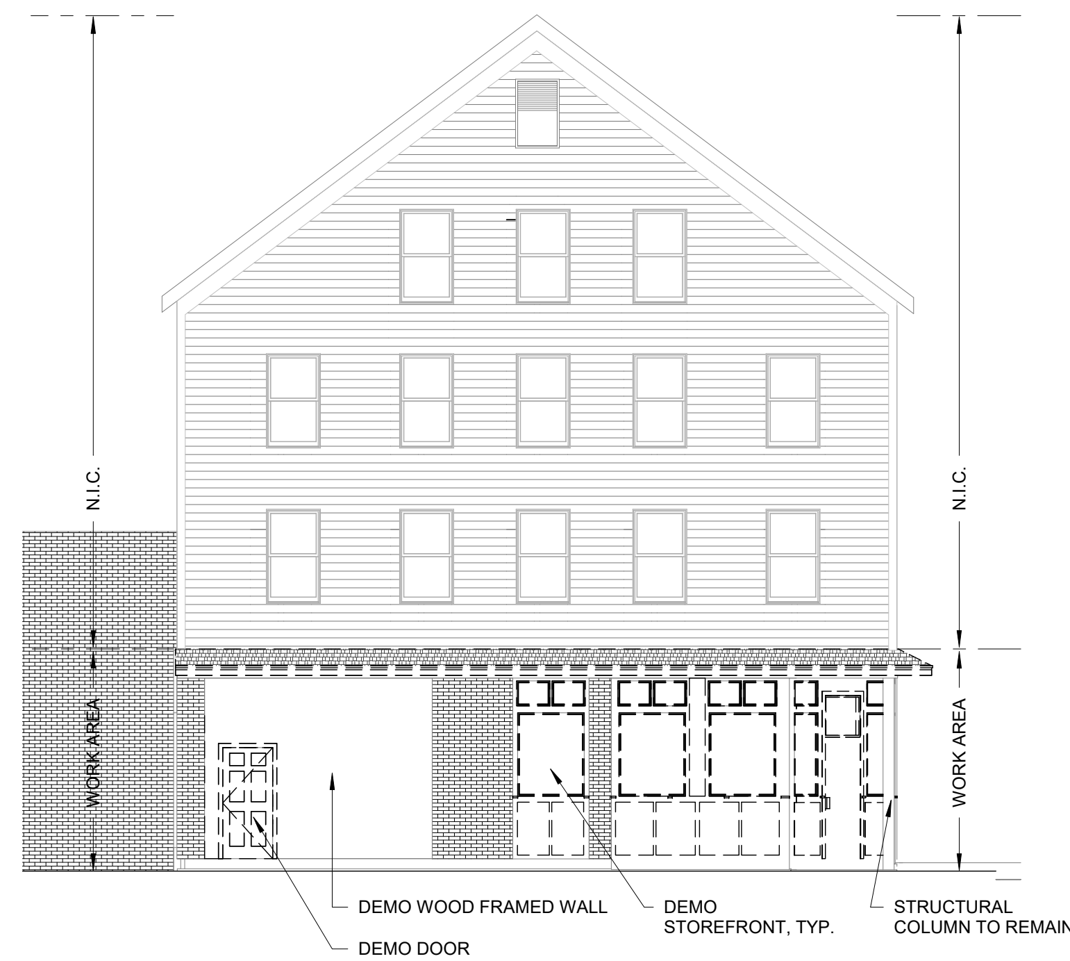
2 | EXISTING SOUTH ELEVATION 1/8" = 1'-0"
