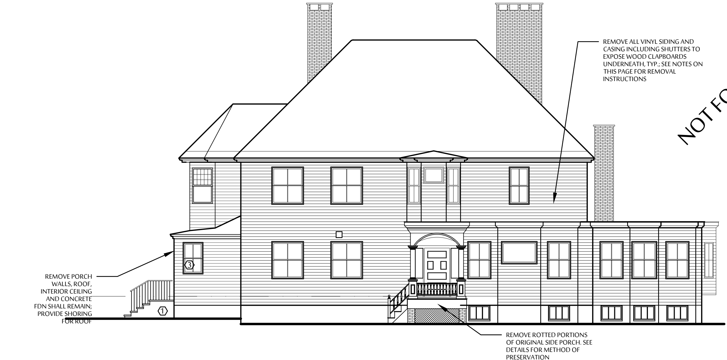
3 SOUTH EXTERIOR ELEVATION 3/8" = 1'-0"
