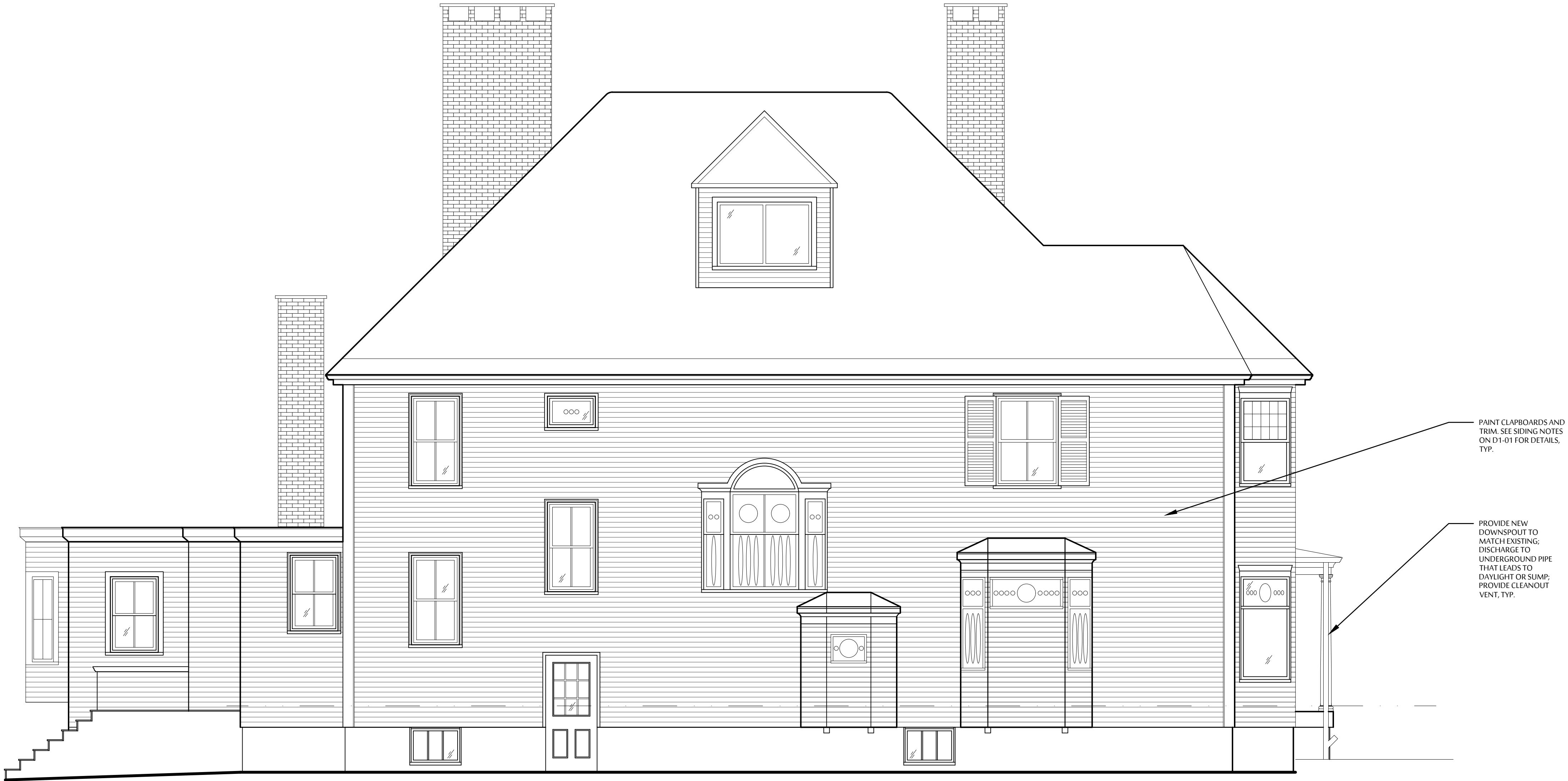
1 NORTH EXTERIOR ELEVATION 3/4" = 1'-0"
