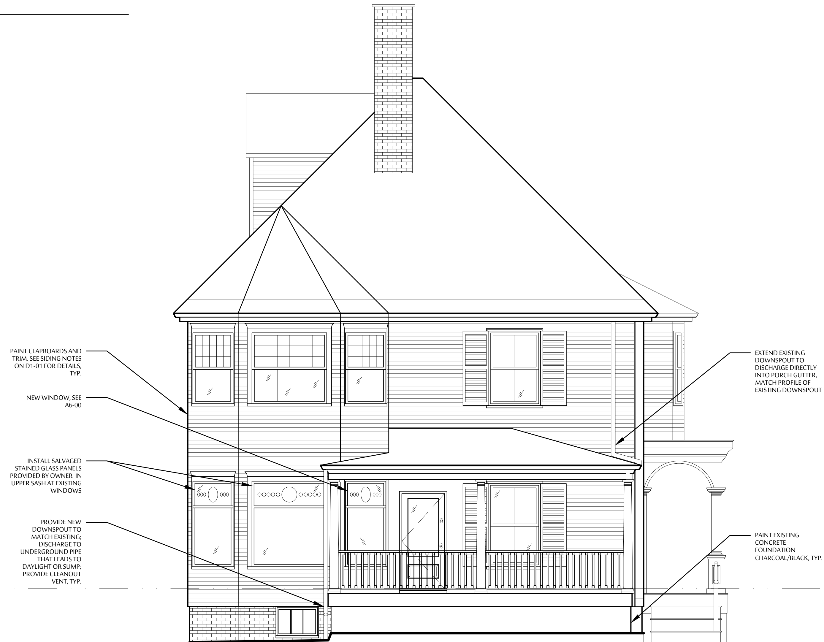
1 WEST EXTERIOR ELEVATION \frac{3}{4}" = 1'-0"
