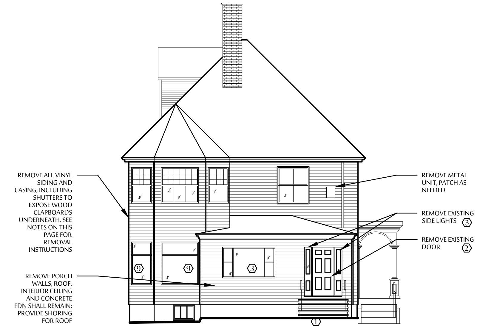
4 EAST EXTERIOR ELEVATION 3/8" = 1'-0"
