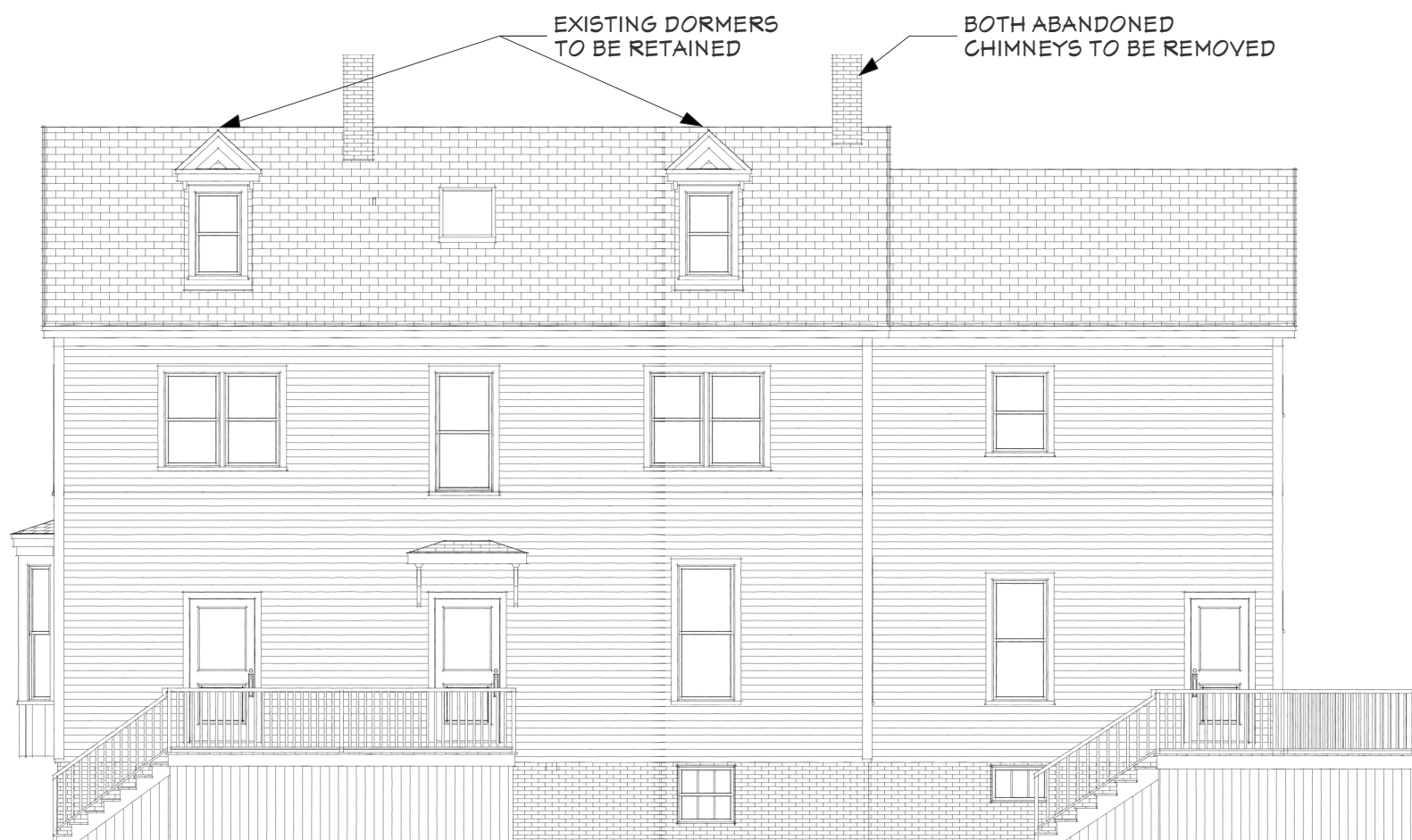
South Elevation (Existing)
