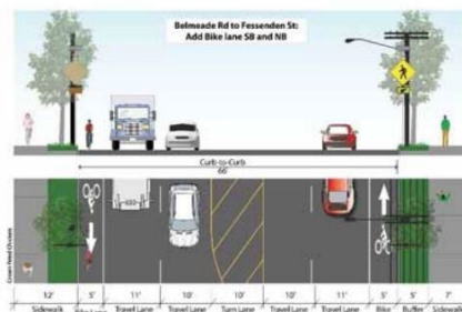
Figure 117. Alternative 1 – Fessenden Street to Belmeade Road
