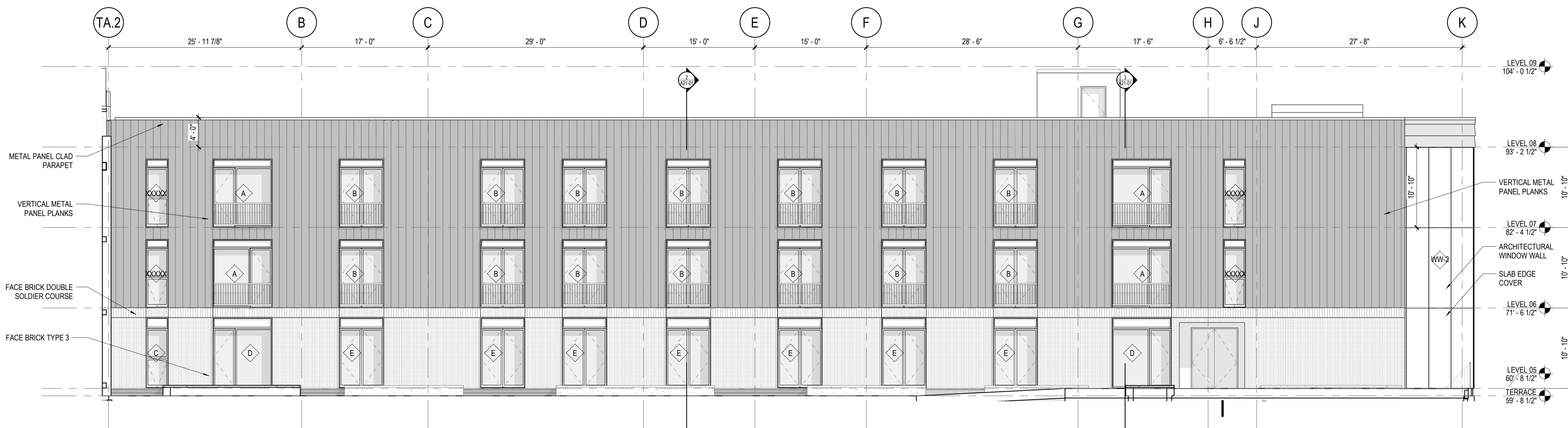
1 COURTYARD 1 ELEVATION - EAST 1/8" = 1'-0"
