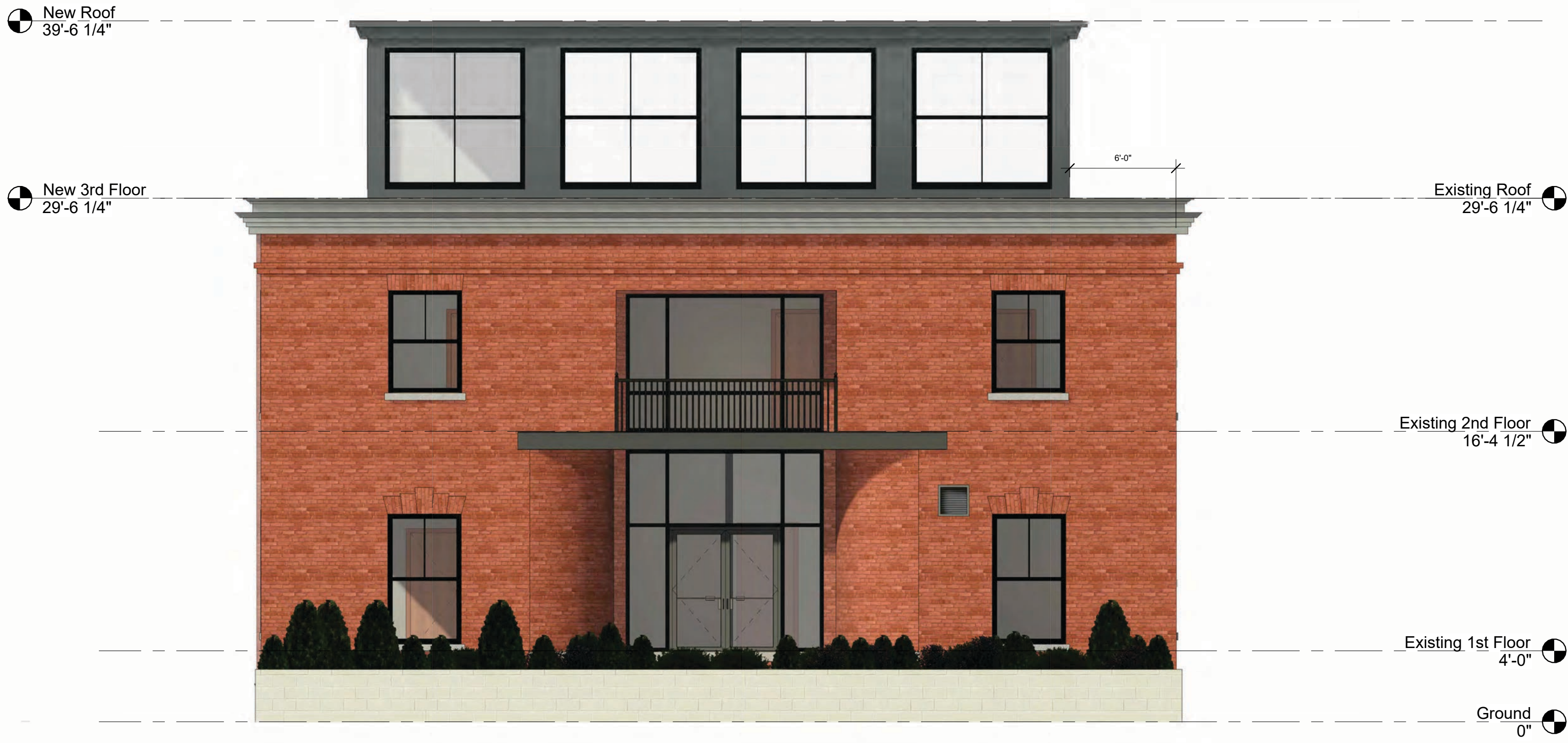
1 | EXISTING BLDG NEW CONSTRUCTION FRONT ELEVATION 3/16" = 1'-0"
