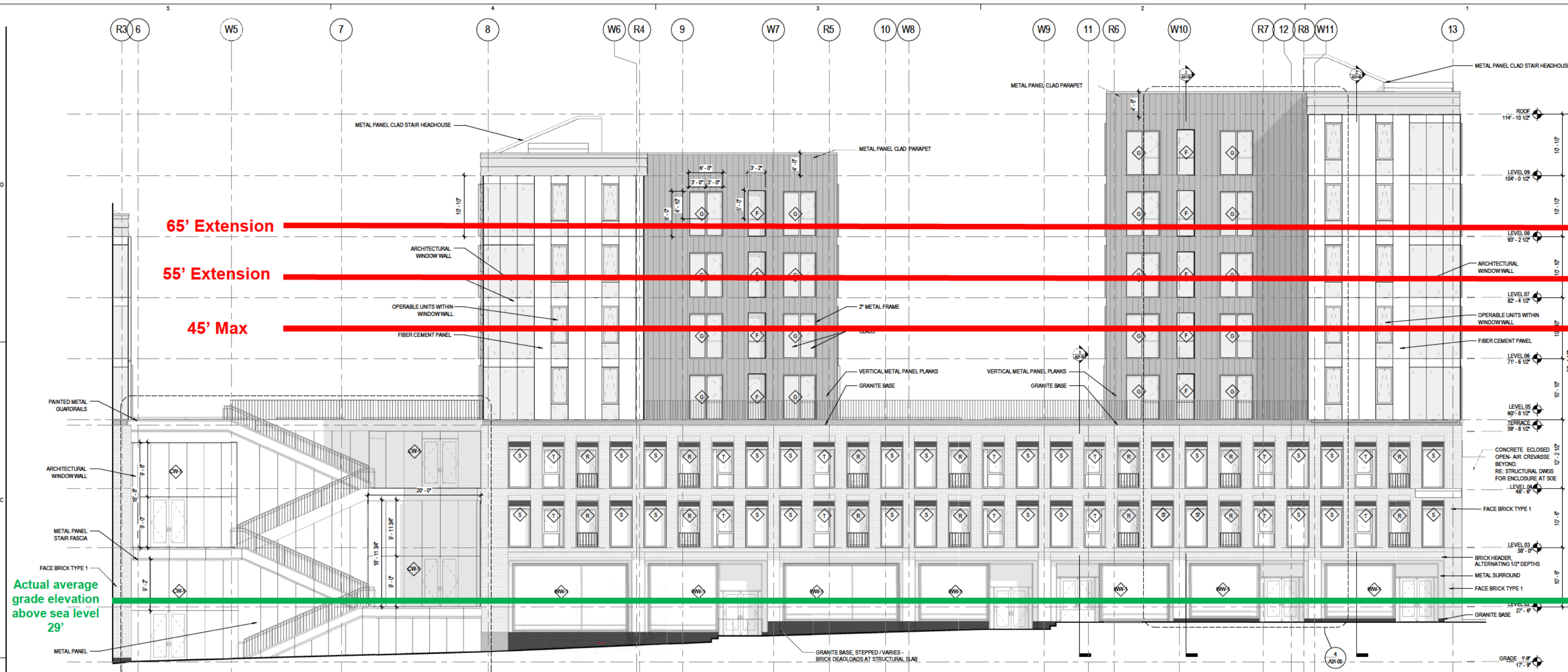
1 OVERALL SOUTH ELEVATION A 1/8" = 1'-0"
