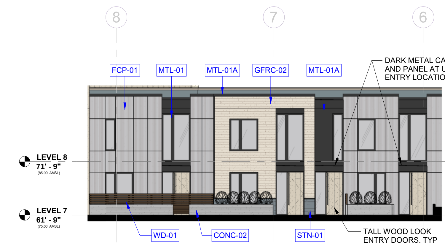
6B ELEVATION - 7TH FLOOR TERRACE ENTRY
