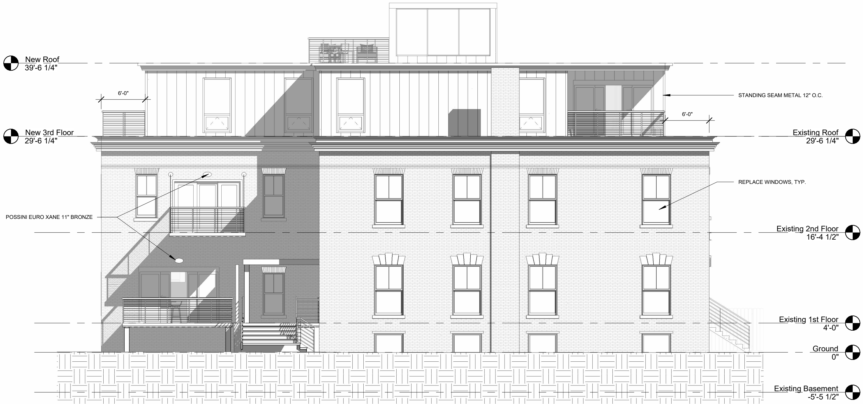
1 | 19 WEST NEW WEST ELEVATION 1/8" = 1'-0"
