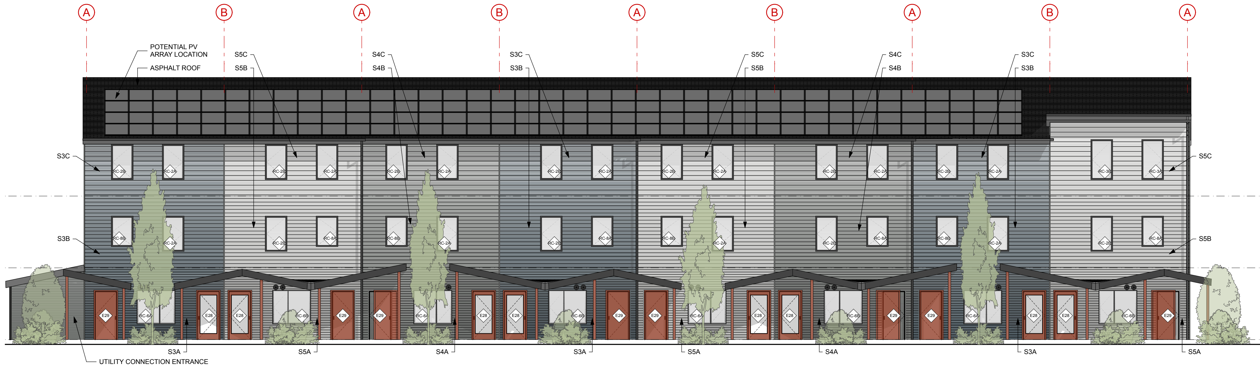
1 ROWHOME, ENTRY ELEVATION SCALE: 1/8" = 1'-0"
