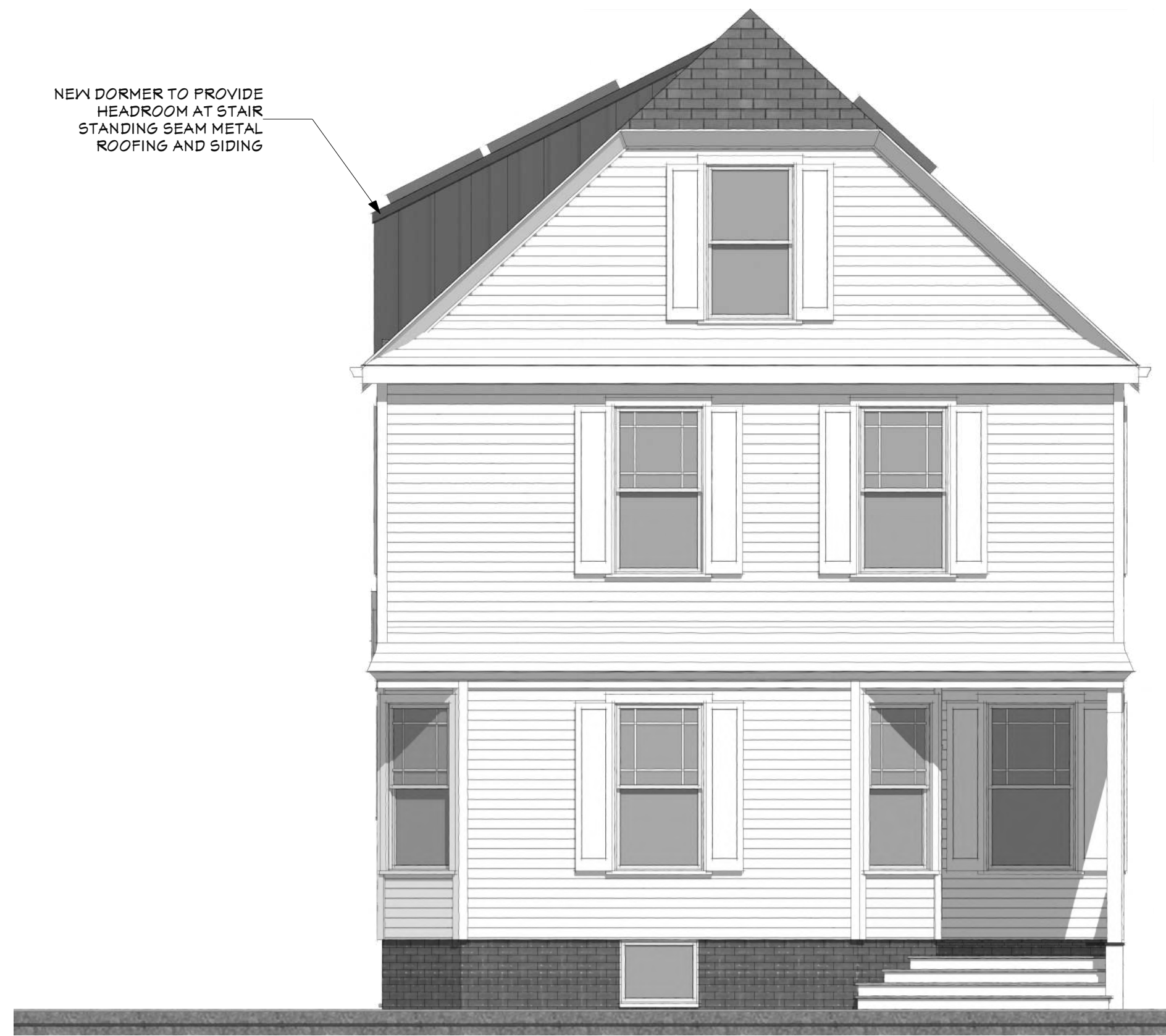
E2 Proposed West Elevation (front) 1/4 in = 1 ft
