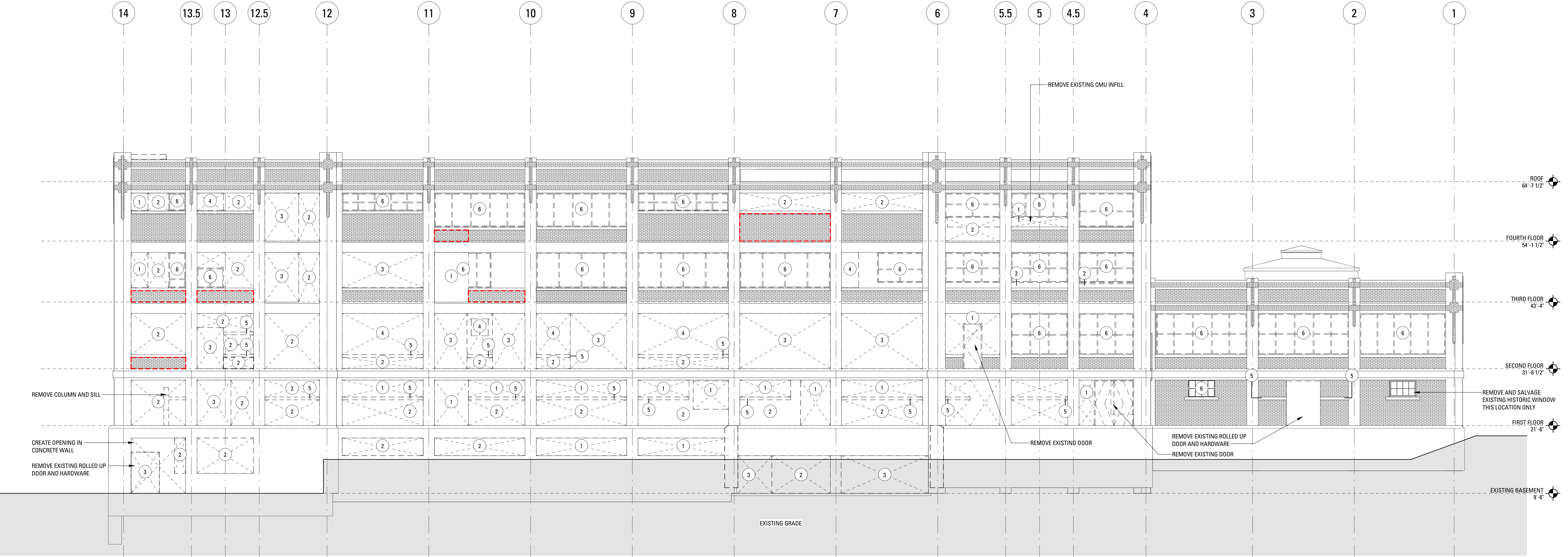
1 DEMOLITION ELEVATIONS - EAST ELEVATION SCALE: 1/8" = 1'-0"
