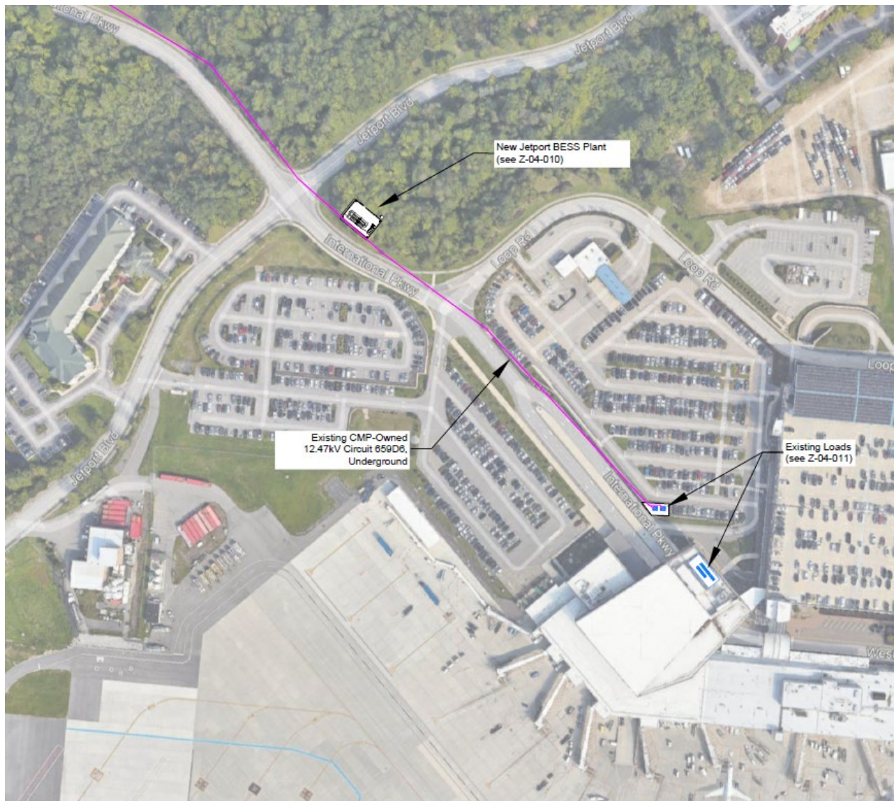
Figure 1. Location of Proposed Battery Storage System
