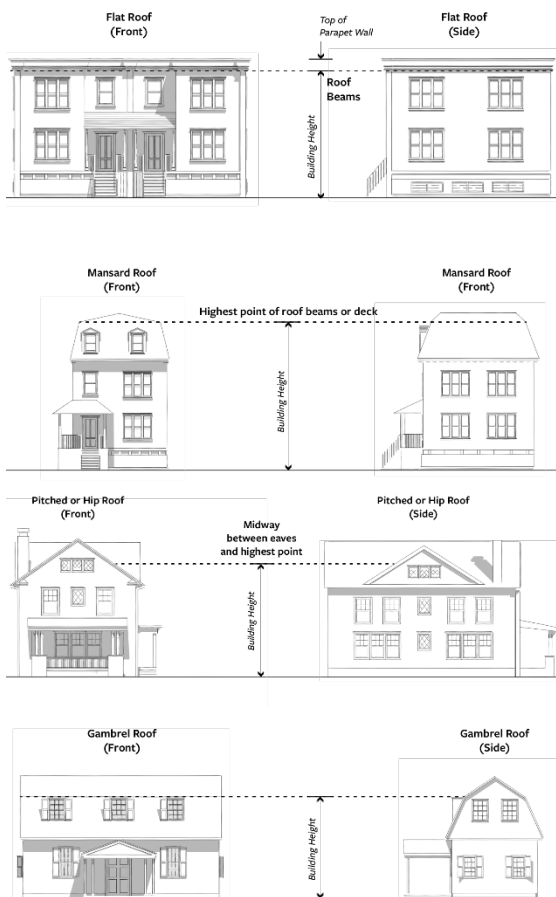
FIGURE 7-E: BUILDING HEIGHT MEASUREMENT
