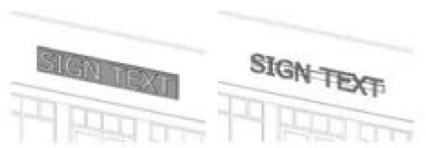
FIGURE 19-B: RACEWAY CABINET EXAMPLES
