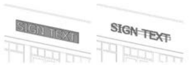
FIGURE 19-B: RACEWAY CABINET EXAMPLES
