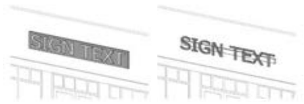
FIGURE 20-B: RACEWAY CABINET EXAMPLES
