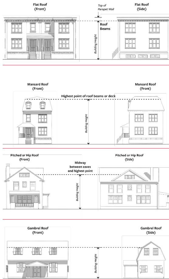
FIGURE 7-E: BUILDING HEIGHT MEASUREMENT
