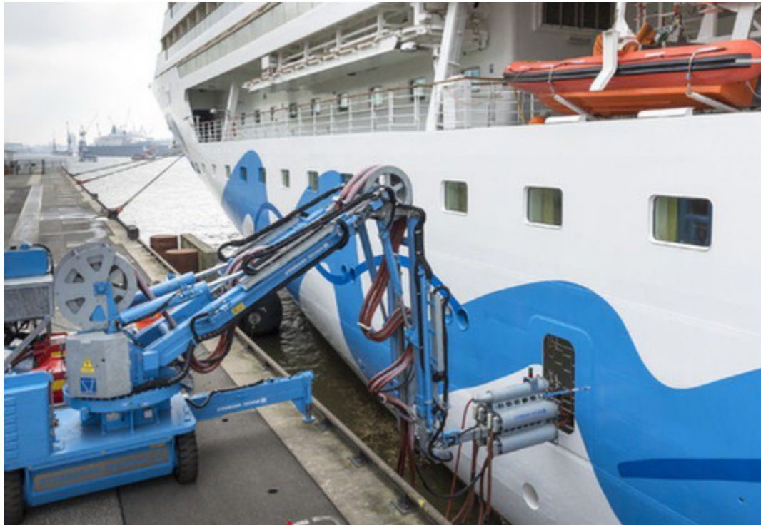
A cruise ship plugging into shore power in Hamburg, Germany (source: CLIA)
