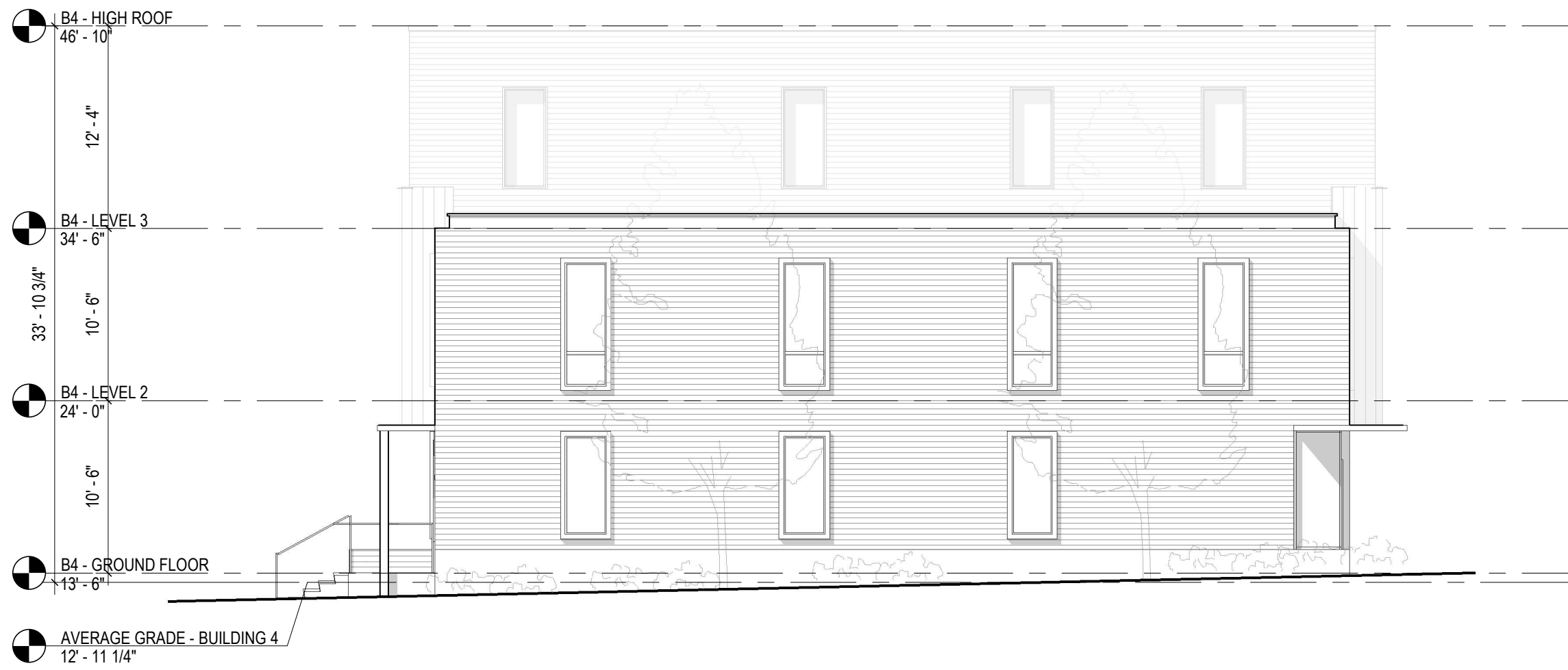
4-BUILDING 4 - EAST ELEVATION
