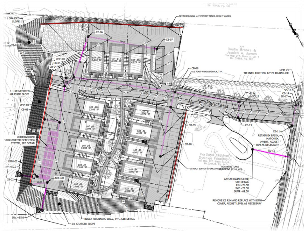
Figure 3: Site Grading Plan
