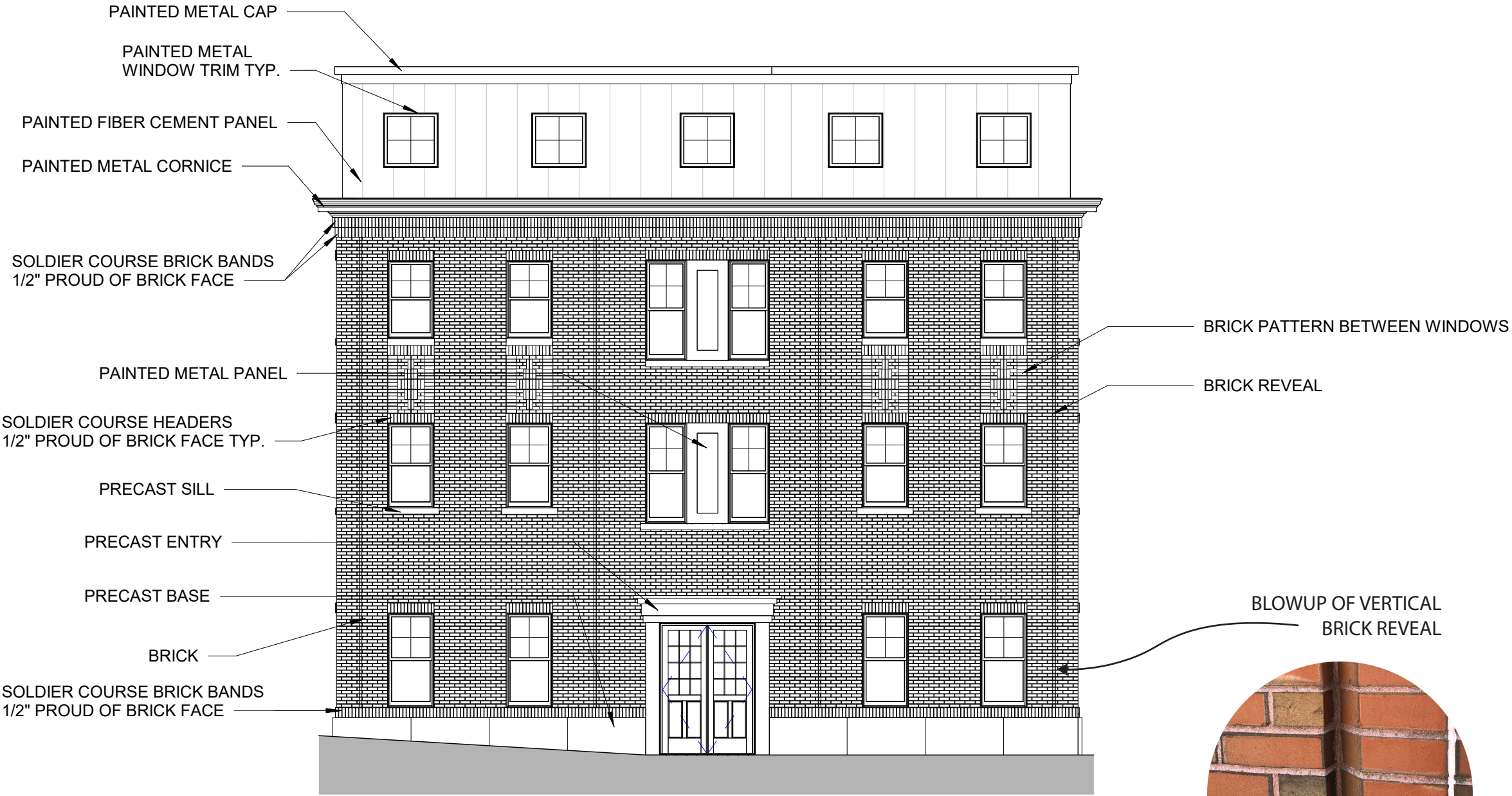
1 | DANFORTH ST ELEVATION 1/8" = 1'-0"
