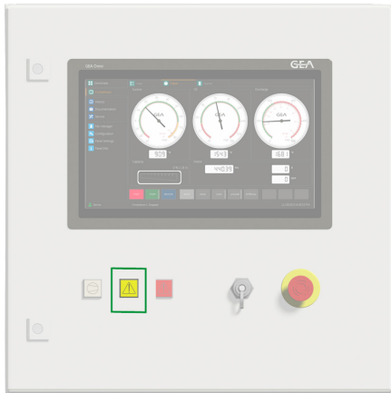
fig.13: Yellow indicator light - screw compressor (Warning)
