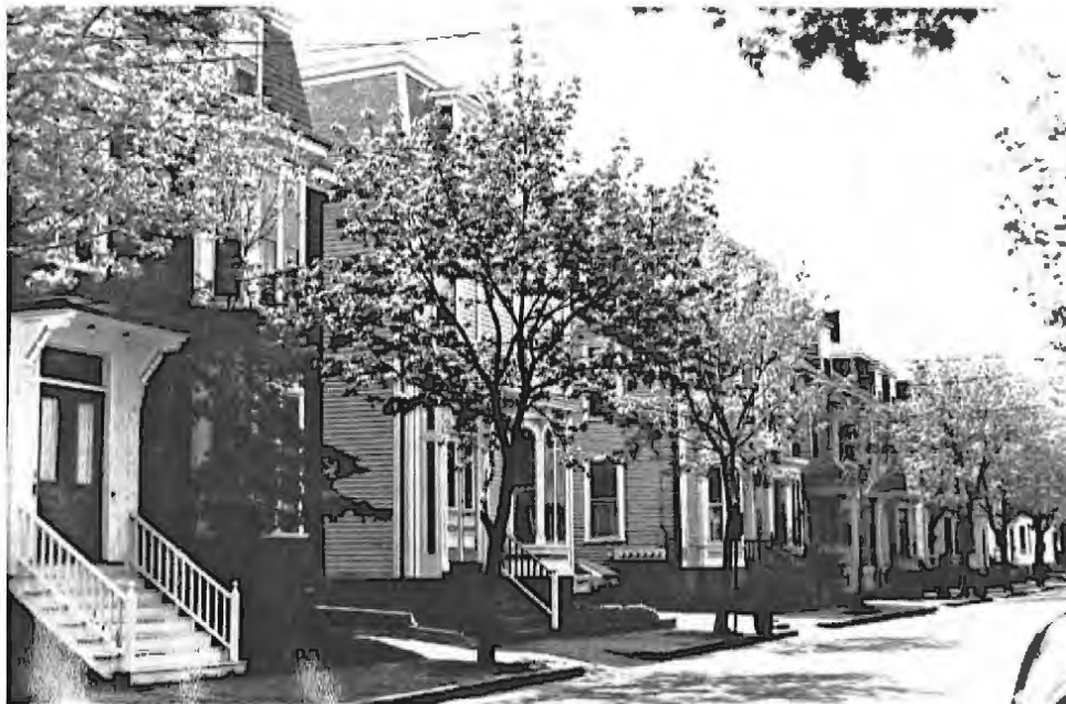
The detached townhouses of Cushman Street represent a case where rooflines are so uniform that a new building inserted into this streetscape would be likely to have a mansard roof with the ridge perpendicular to the street. While a dramatically different roofline would not be ruled out, such a design would need to be carefully considered and justified as to its compatibility.
