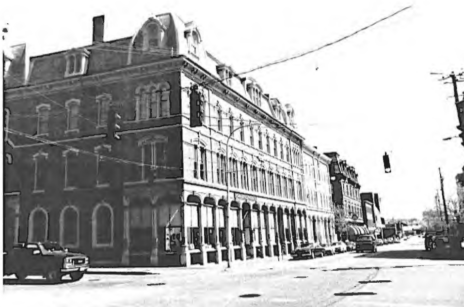
The proportion of Victorian commercial buildings was set by many factors resulting from land use and sale patterns, limitations of building technology, etc. This view of commercial blocks on Middle Street shows a remarkable row of large three-story buildings that are very similar in scale and proportion. Such a strong pattern should be a design determinant for any new construction proposed for adjacent sites.
