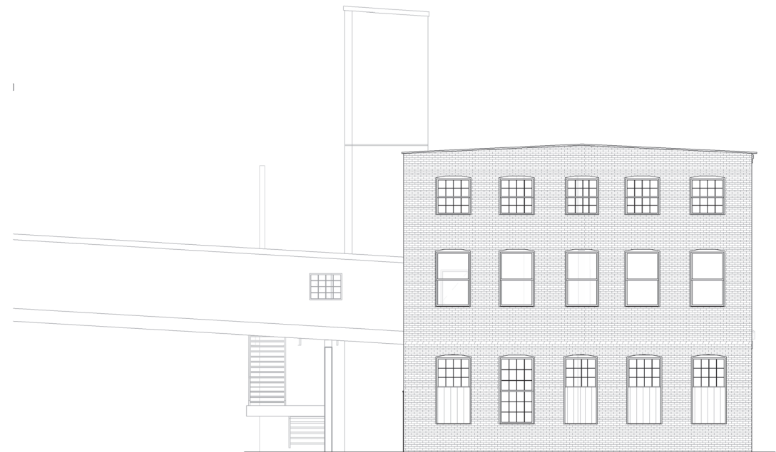
2 BUILDING 6 - EXISITING WEST ELEVATION SCALE: 1/8" = 1'-0"
