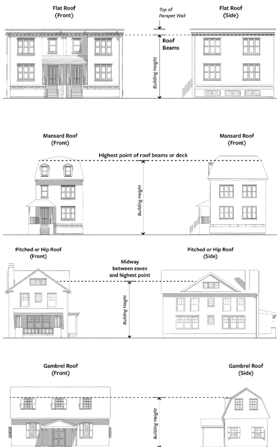
FIGURE 7-E: BUILDING HEIGHT MEASUREMENT
