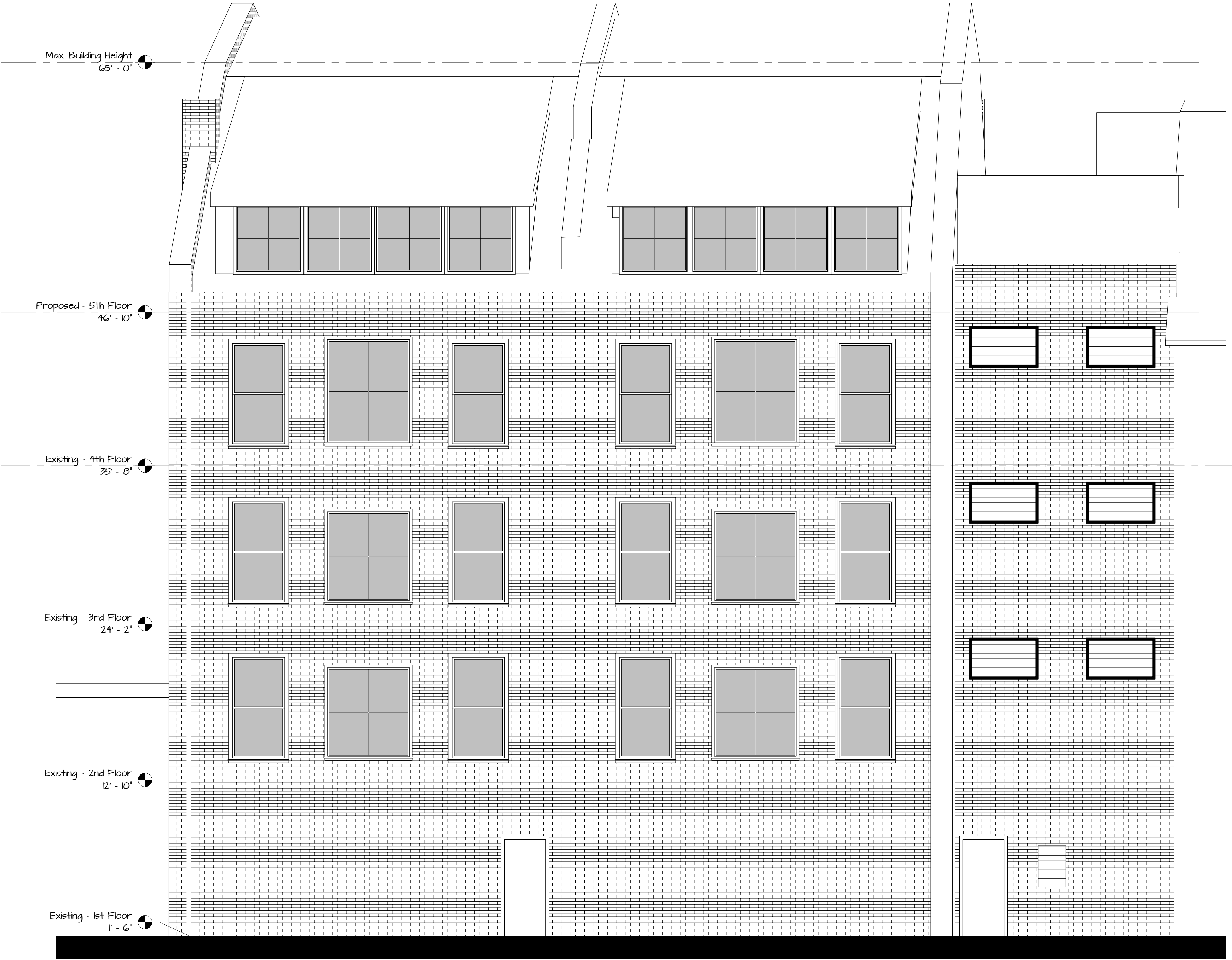
EXISTING REAR ELEVATION 1/4" = 1'-0"
