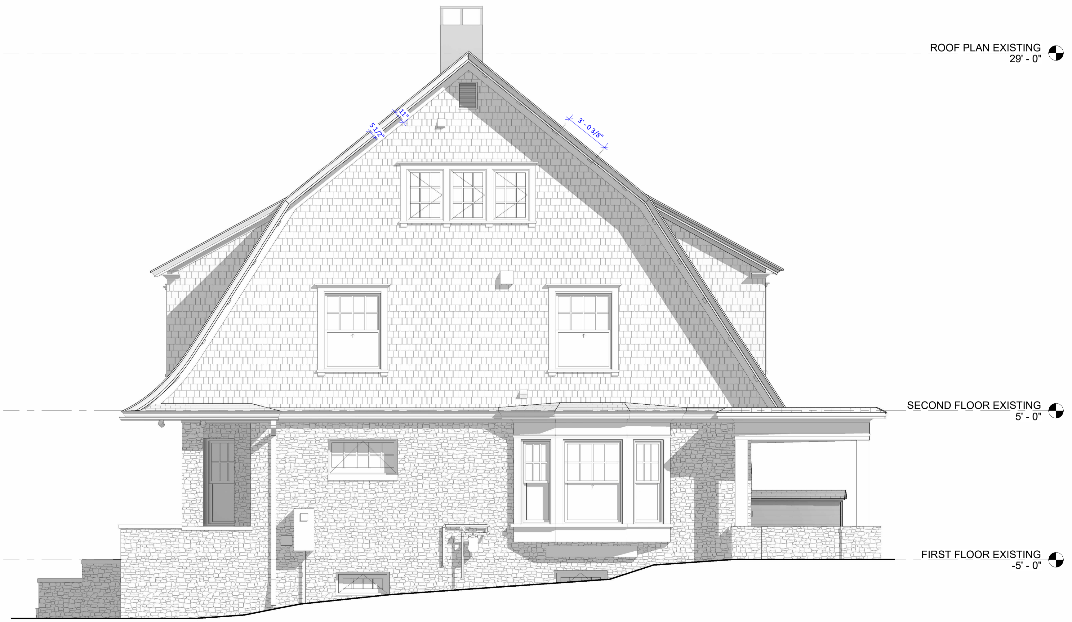
2 EAST ELEVATION - EXISTING A201 SCALE: 1/4" = 1'-0"
