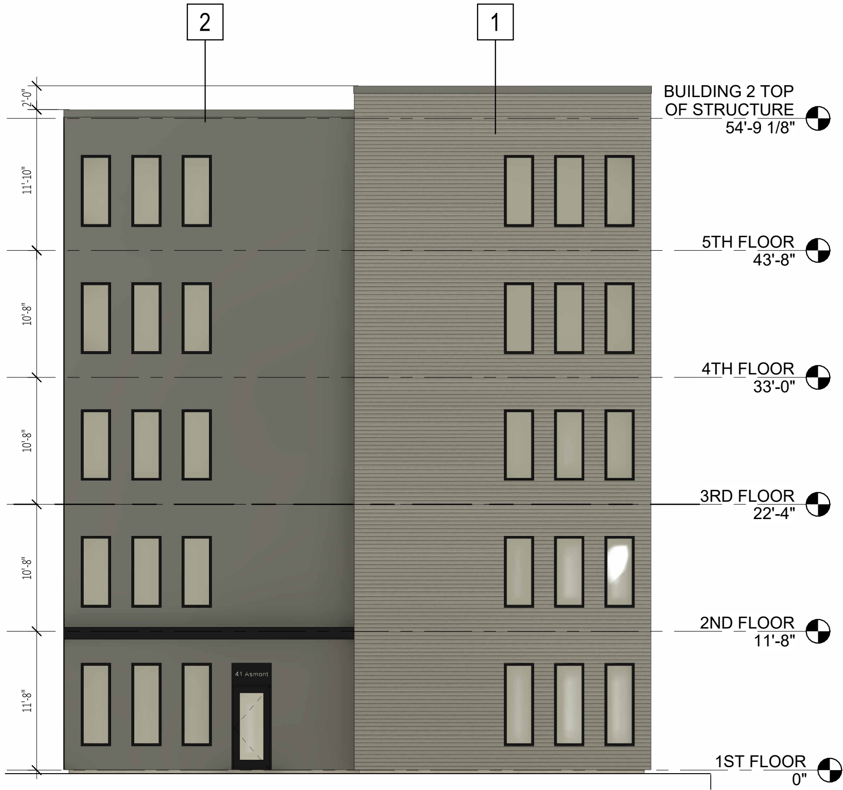
4 | SOUTH ELEVATION - BUILDING 2 1/8" = 1'-0"
