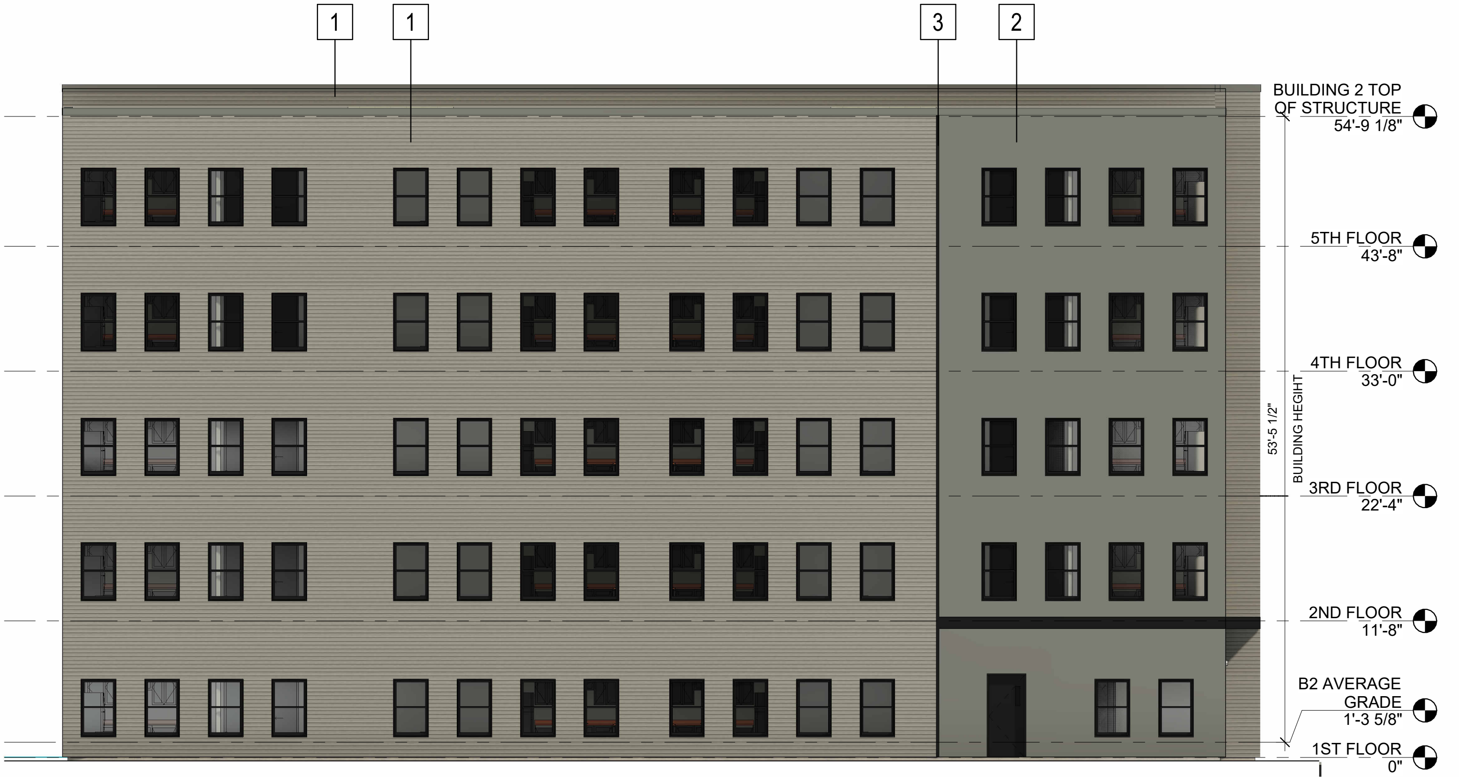
2 | WEST ELEVATION - BUILDING 2 1/8" = 1'-0"
