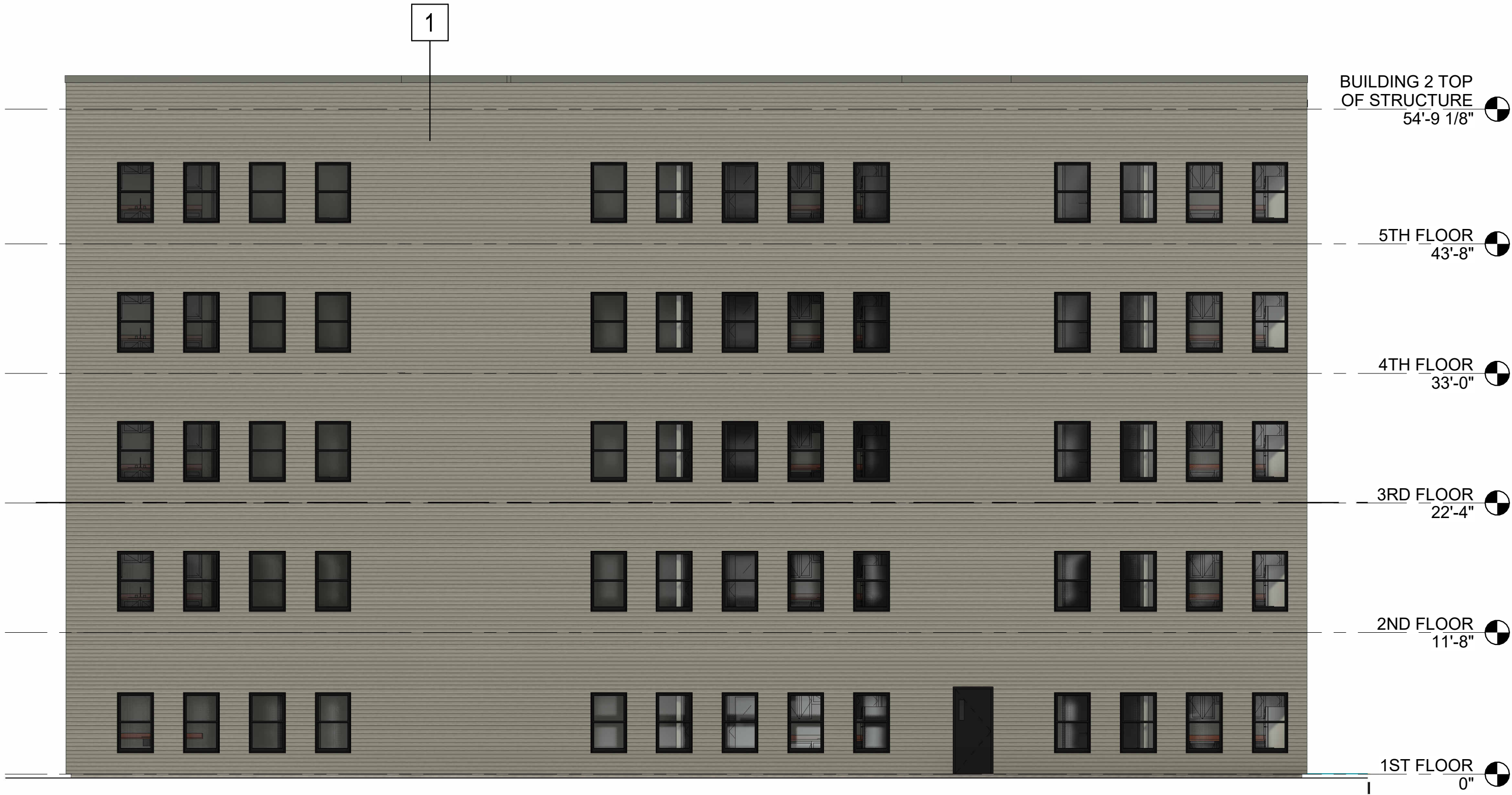
1 | EAST ELEVATION - BUILDING 2 1/8" = 1'-0"
