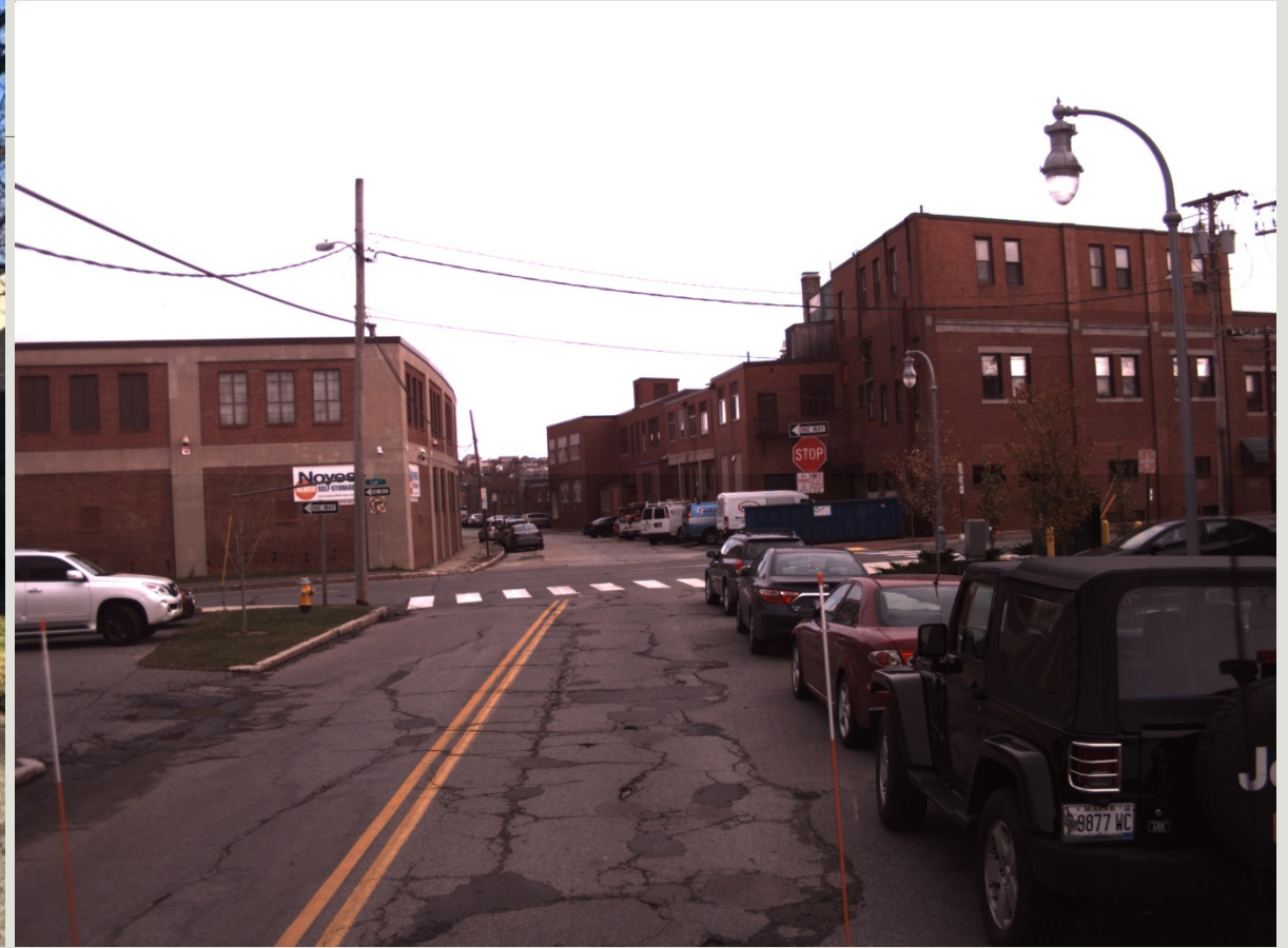
Kennebec Street – PCI = 42; ranked Poor Mill/fill treatment recommendation
