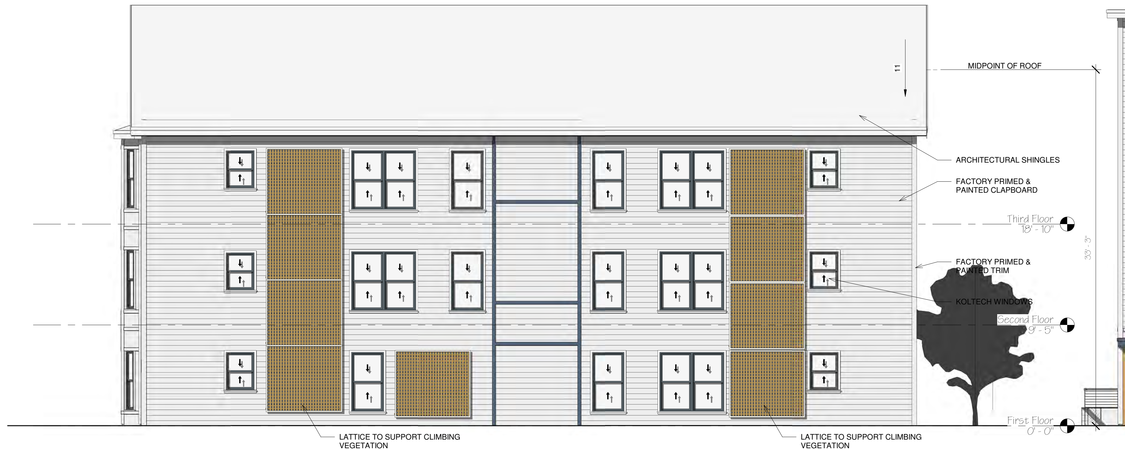
C East Elevation 126 North 3/16" = 1'-0"
