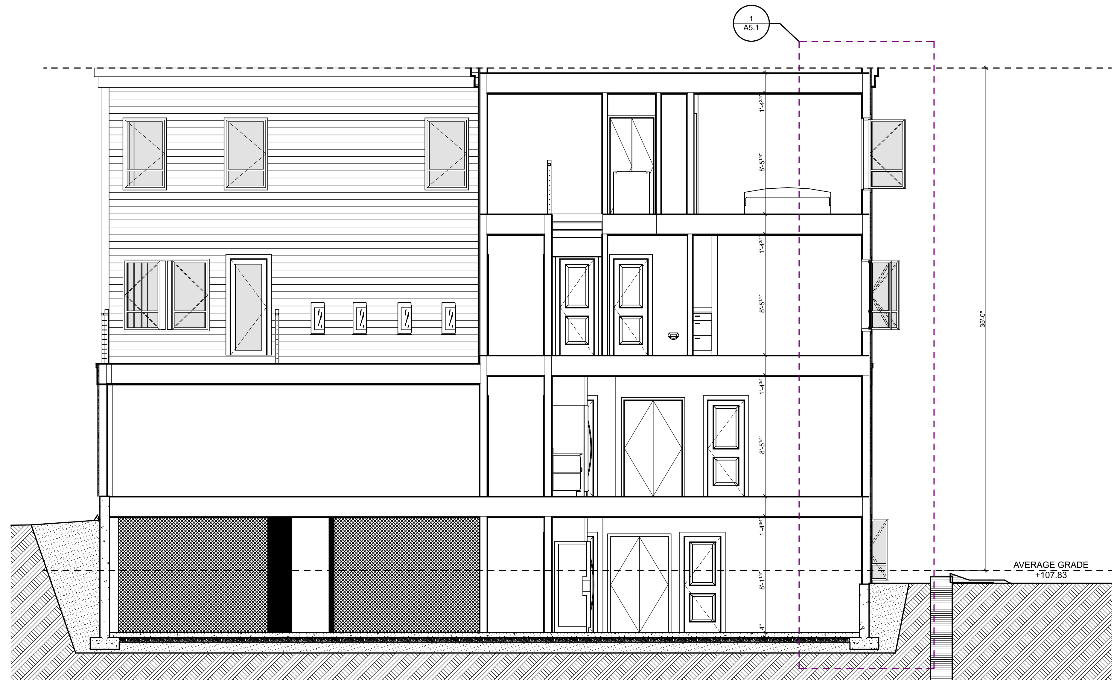
1 A3.1 N/S BUILDING SECTION SCALE: 1/4" = 1'-0" 0 2' 4' 8'
