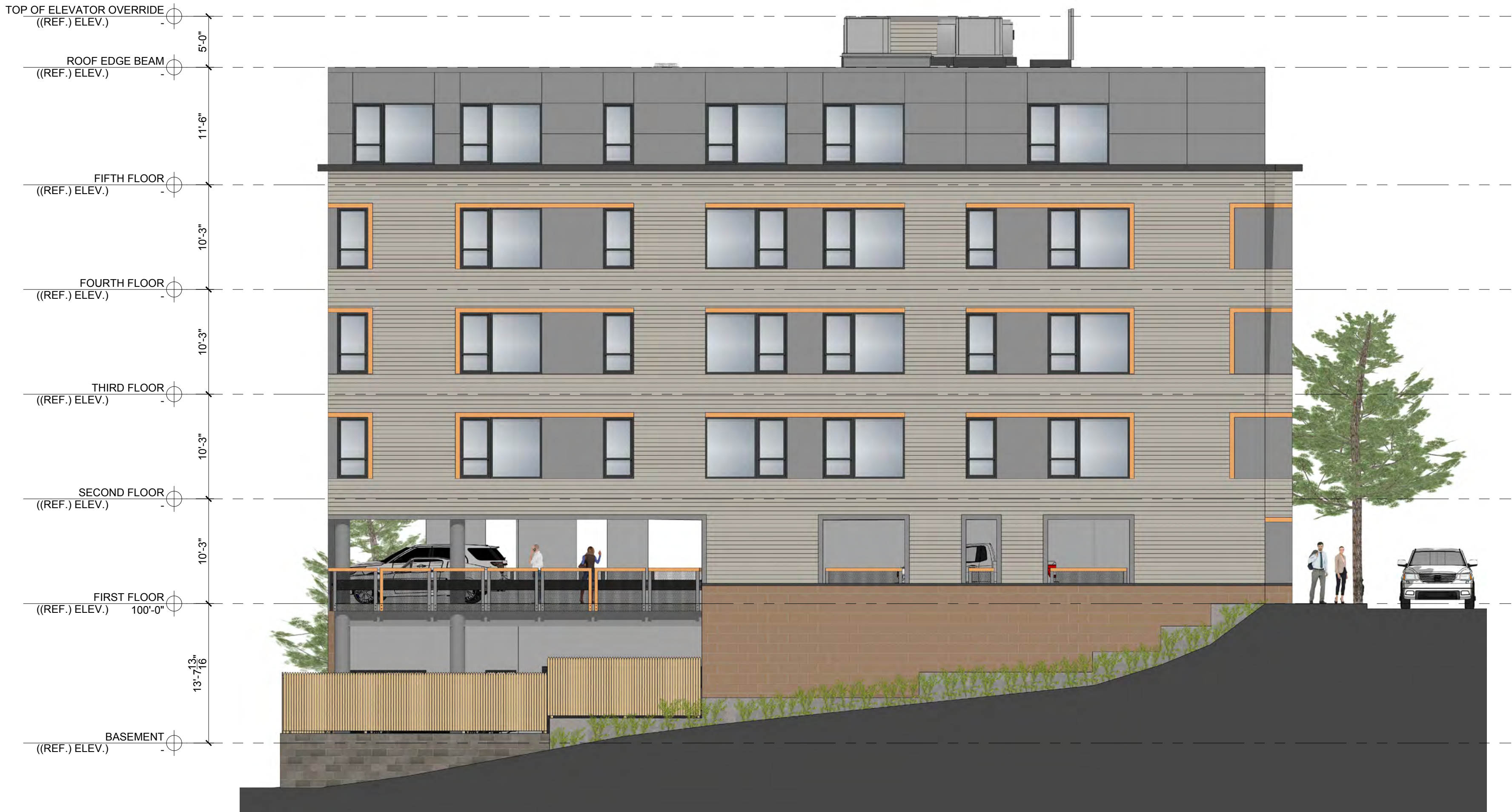
1 VALLEY STREET SOUTH ELEVATION 1/8" = 1'-0"
