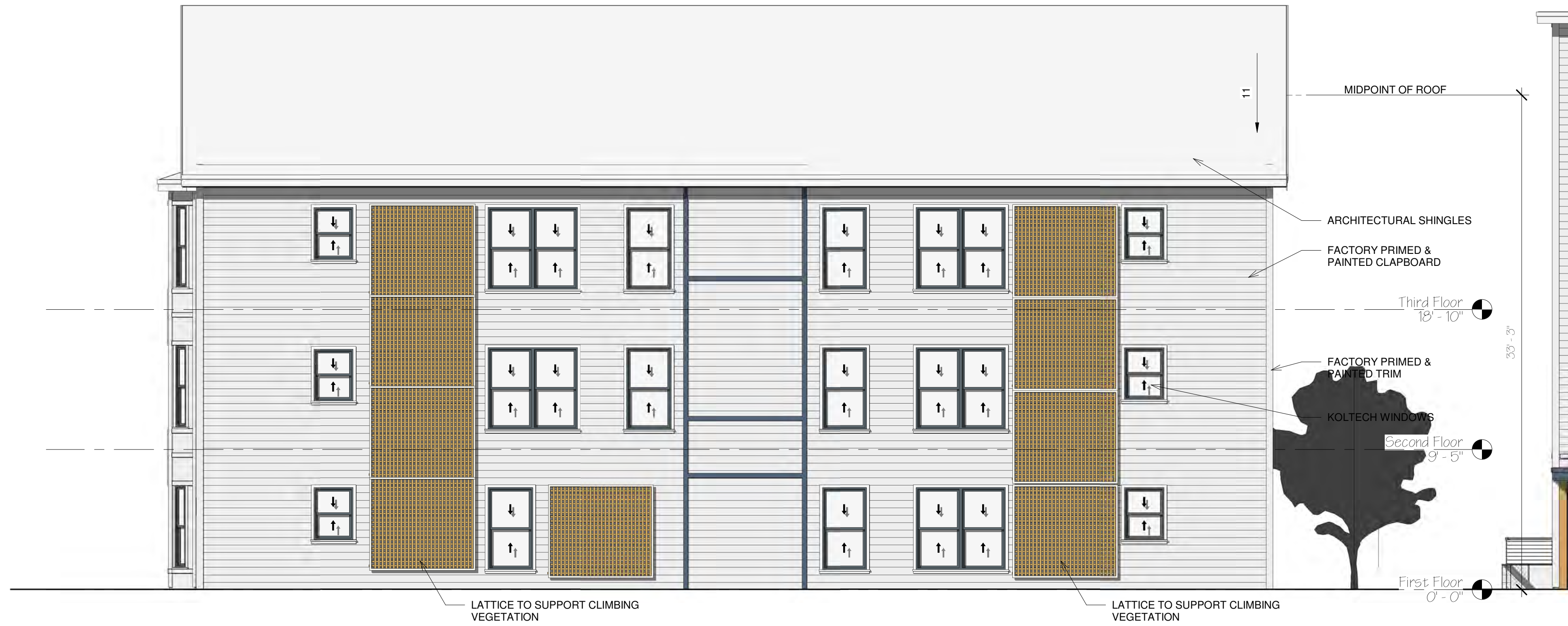
C East Elevation 126 North 3/16" = 1'-0"
