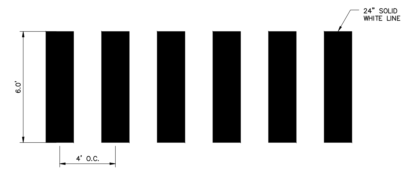
CROSSWALK WITH LONGITUDINAL LINES
