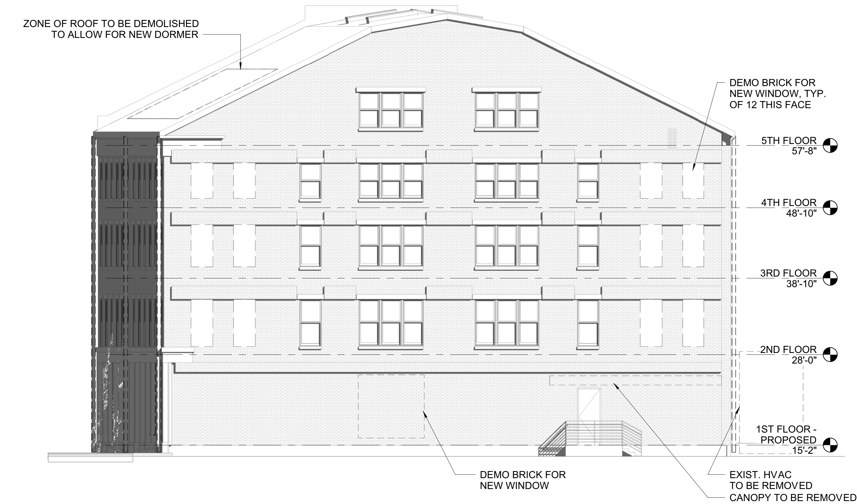
4 | EAST ELEVATION - EXIST/DEMO 1/8" = 1'-0"
