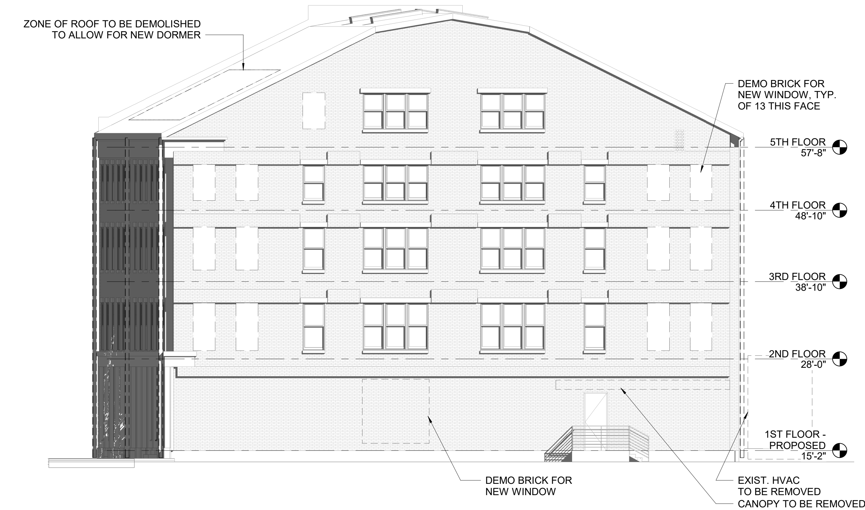
4 | EAST ELEVATION - EXIST/DEMO 1/8" = 1'-0"
