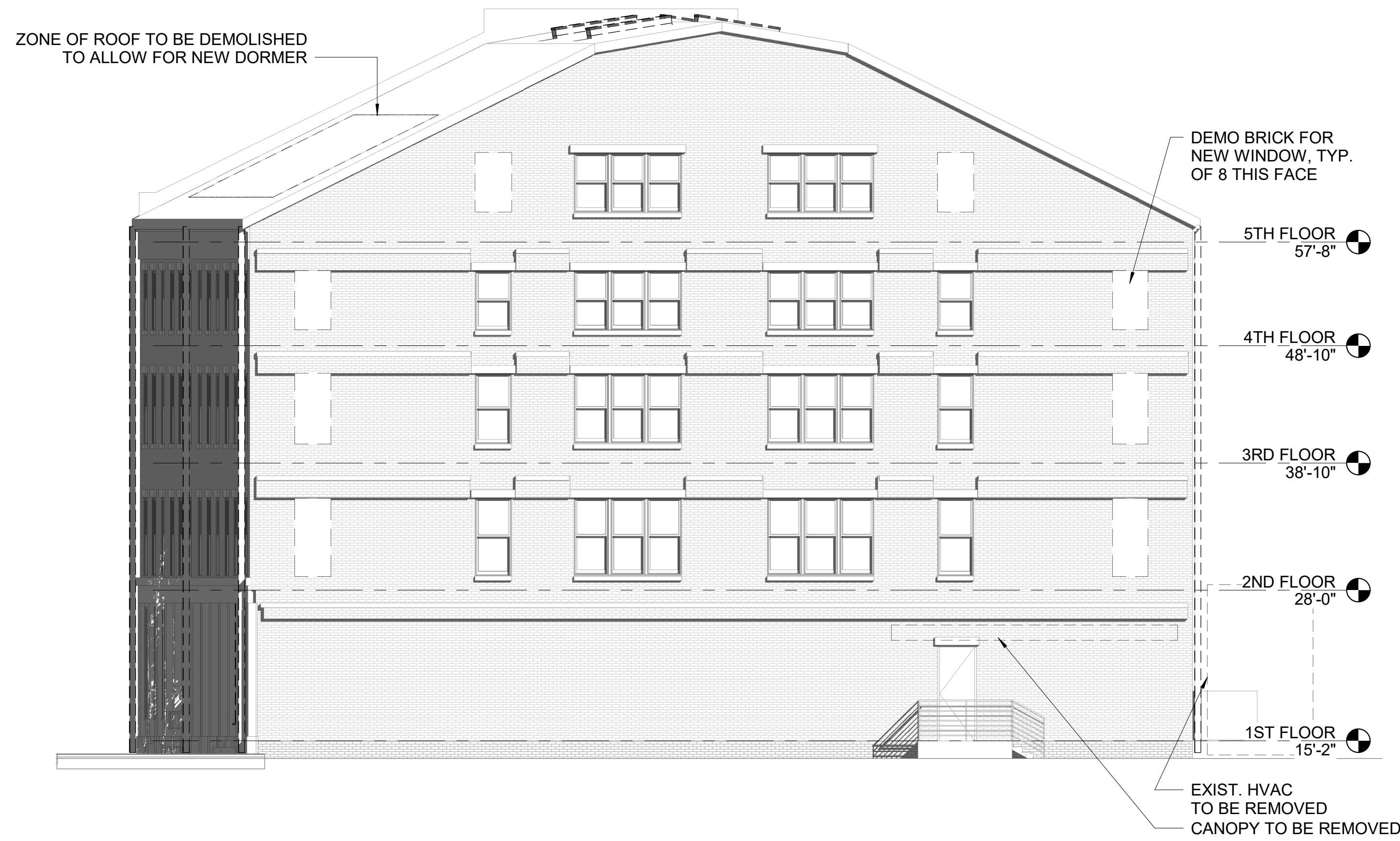
4 | EAST ELEVATION - EXIST/DEMO 1/8" = 1'-0"
