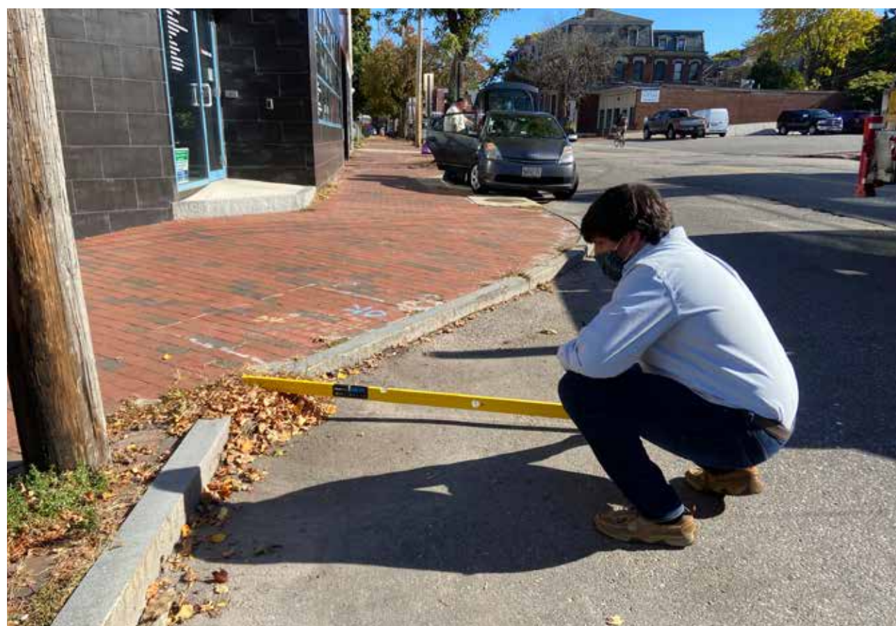
Accessibility and grading- curbline extention in this location could allow for ADA accessible sidewalk
