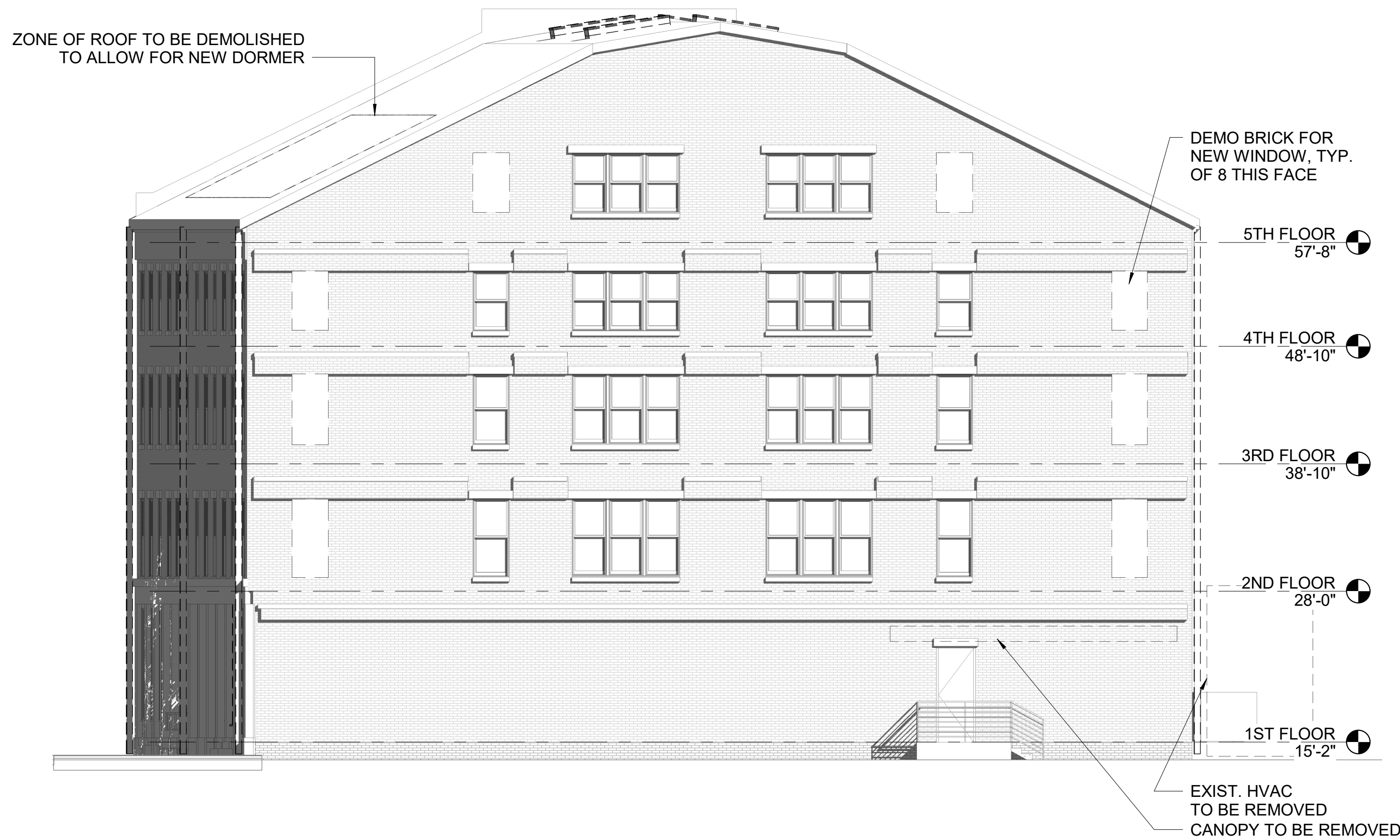
4 | EAST ELEVATION - EXIST/DEMO
